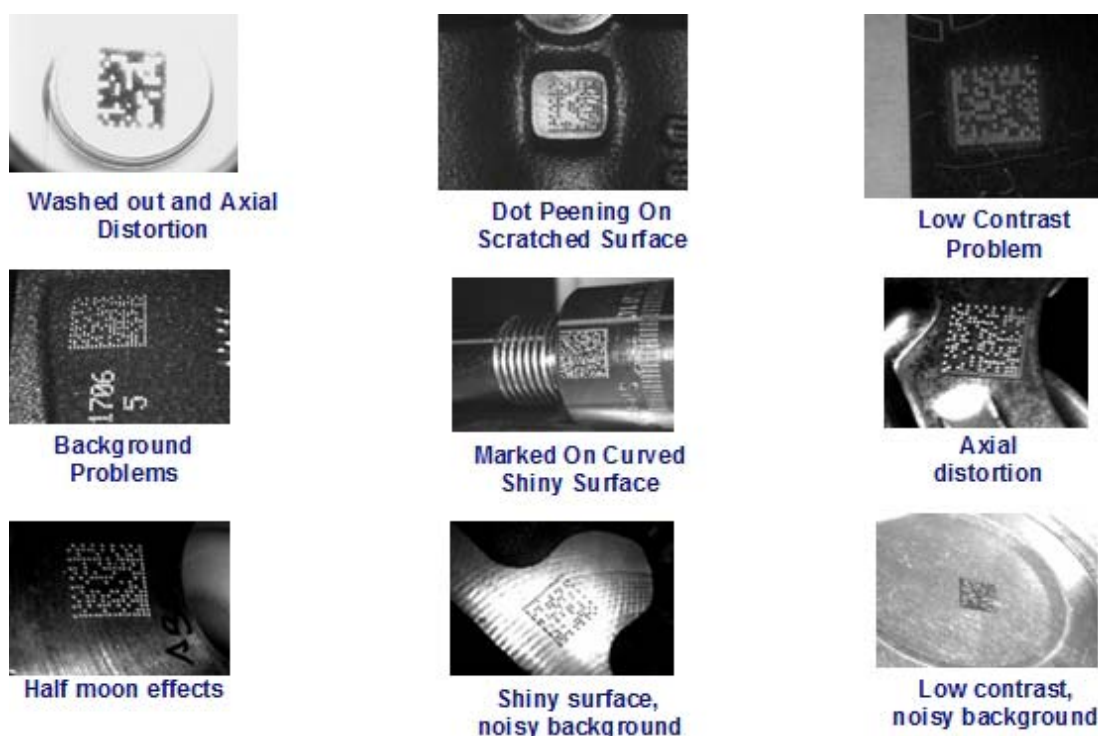
Figure 7 – Problematic Direct Part Marking Examples
