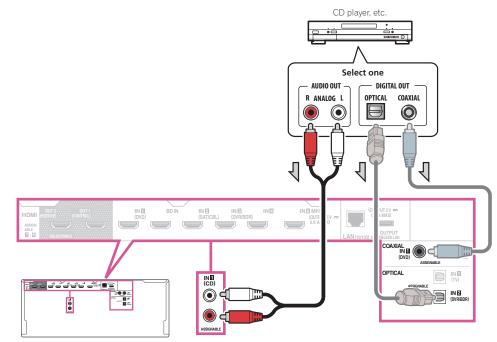
• If your turntable has line-level outputs (i.e., it has a built-in phono pre-amp), connect it to the **ANALOG IN 1** (CD) inputs instead.
