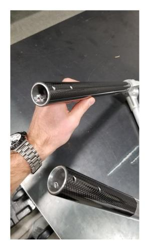
Tube inserts machined down and ground to fit inside aluminum tube
