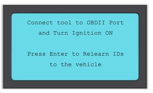
Plug in the OBD II cable and then turn only the ignition on, you should not need to start the engine. If you cannot find the OBD location right away, please use the "View Vehicle Information" menu and select "View Vehicle Info." the tool displays now where the OBD is positioned.
