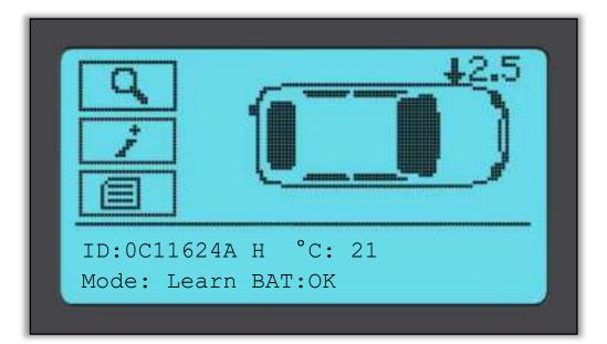
The arrow will then automatically move on to the next wheel position (Right Front, Right Rear and then Left Rear), and the pressure will be displayed against the previous wheel position, in Bar or PSI as selected in Settings.
