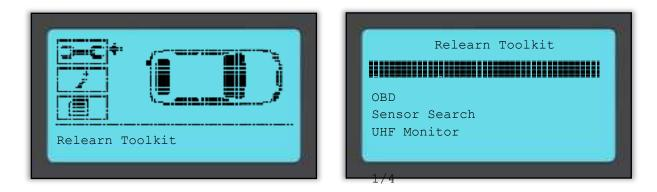
In this case the left front sensor has already been read, but needs to be replaced. After reading use the Down Arrow to navigate to the 'Relearn Toolkit' then 'Program Sensor' and select the programmable sensor you would like to use.
