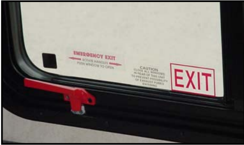
Figure 13-1. Emergency Exit Window
