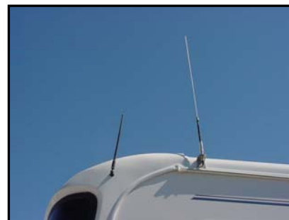
Figure 4-19. CB Antenna Installation
