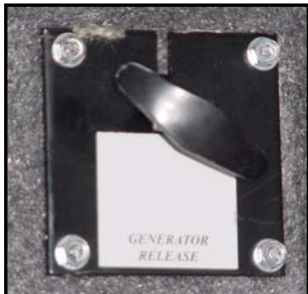
Figure 7-17. “Pull” Cable for Generator Release
