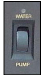
Fig. 11-5. Water Pump Switch
