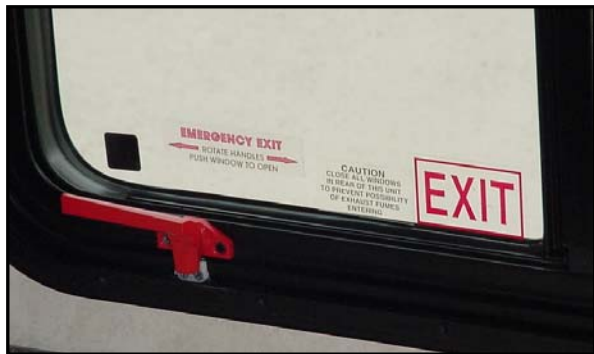
Figure 2-7. Emergency Exit Window
