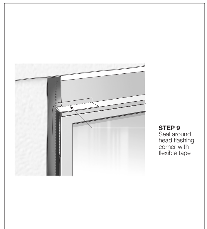
FIGURE 38 INSTALLATION OF WINDOW
