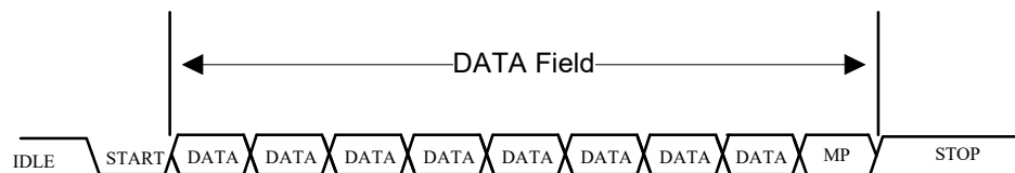
Figure 23-28. UART MP Address and Data Frame
