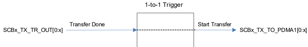
Figure 29-8. Example of 1-to-1 Trigger
