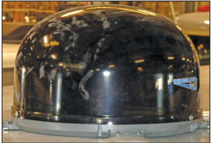
Figure 7-1: The dome satellite on top of the motorhome can be raised allowing easy access to change switches to a new satellite provider.
