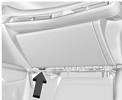
Interior Power Outlet
