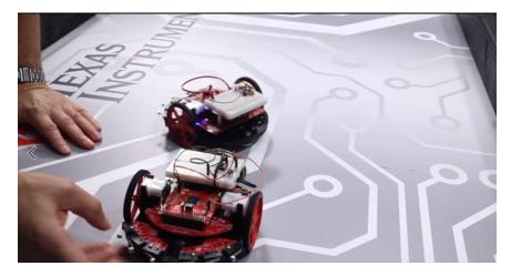
Figure 13. The robots with the microphones will dance to the sounds generated in the robot with the speaker.
