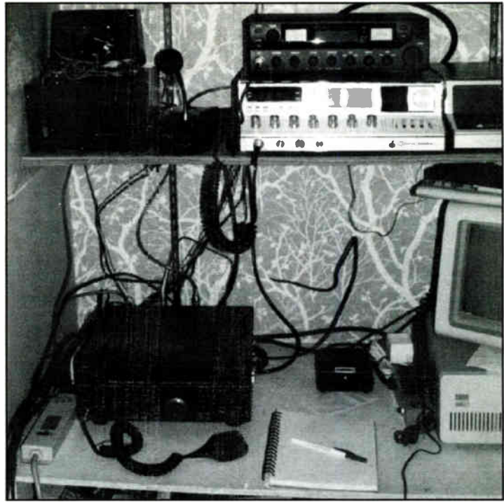
Amid a rat's nest of wires at a secret location in the Northeast, a freebander's tools of the trade: a Cobra 2010 (top right) on top of a Cobra 2000, and (at lower left) a Kenwood TS-850. At upper left, a 20-amp power supply and antenna control box.
