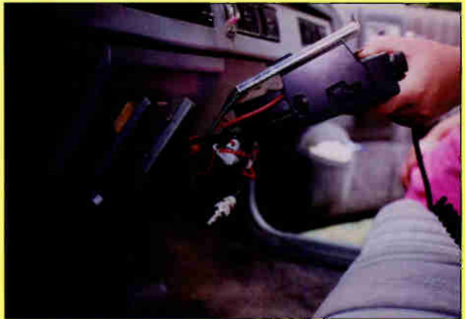
A typical slide-mount is an excellent way to install your CB. All the connections, including the coax, are connected to the part that remains in the vehicle. The other part of the slide-mount attaches to your radio. When you park your vehicle, simply slide out the transceiver and take it with you. (Photo by Harold Ort)
