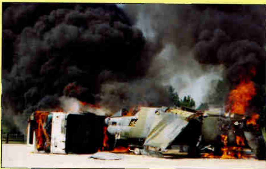
Fire rages from a simulated crash between a mass transit bus and military attack fighter. (Courtesy Richard Feinberg, University of Oklahoma REACT)
