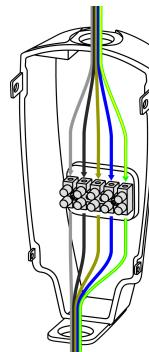
The following illustration shows an example of the wiring for the low profile bracket.
