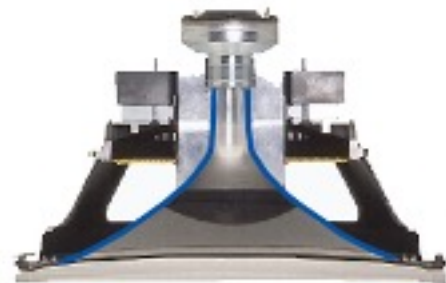
CONTROL 322C/CT CONSTANT DIRECTIVITY CO-AXIAL DRIVER, SHOWING HORN CONTOUR (BLUE LINES) AND NEODYMIUM COMPRESSION DRIVER
