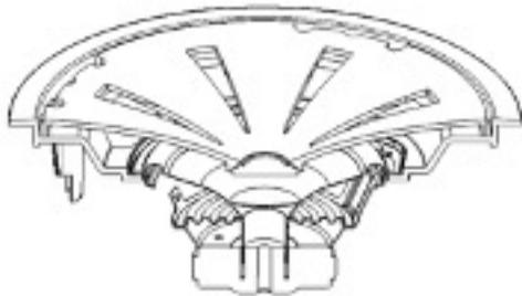
FIGURE 9 WIDE DISPERSION ORBI ON WOOFER
