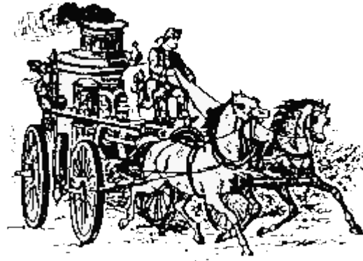
First Company of paid Fire Department to go "in service" was Engine Co. 1, located in lower Manhattan at 4 Centre Street. Apparatus was horse-drawn Amoskeag steam-powered pumper which was same type issued to later companies. Wheels were steel rimmed.
