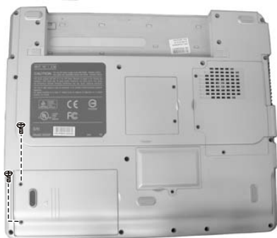
Figure 2-9 Remove the HDD cover
