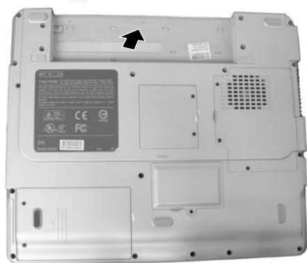
Figure 2-2 Push the keyboard cover
