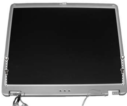
Figure 2-24 Remove LCD frame
