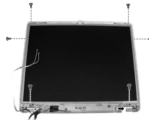
Figure 2-25 Remove LCD panel
