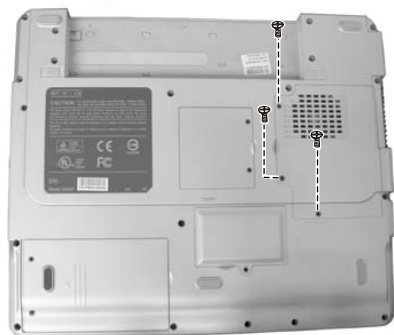
Figure 2-6 Remove the CPU compartment cover
