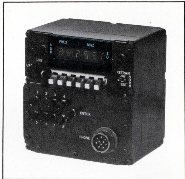
This Hoffman Model VCS-801 control box contains 5/16-in. character, incandescent filament DIP readouts. It displays a six-digit frequency plus a decimal point in the 2.0000 to 29.9999 Mhz range and uses a 22-bit core memory to achieve non-volatility.
