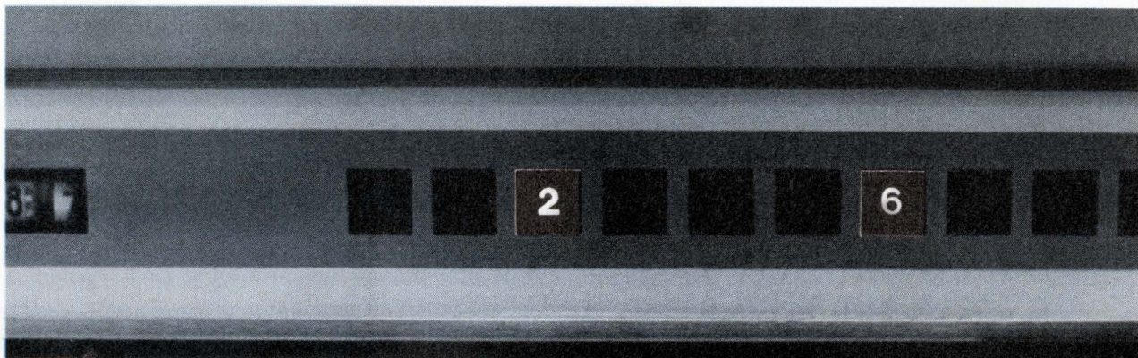
Convergence. This detail of the electromechanical counter of a Xerox 1000 copier shows the static backlit numbers. When the left-hand number, representing copies produced, reaches parity (coincides) with the right hand number, representing copies requested, the copying mode automatically shuts off.
