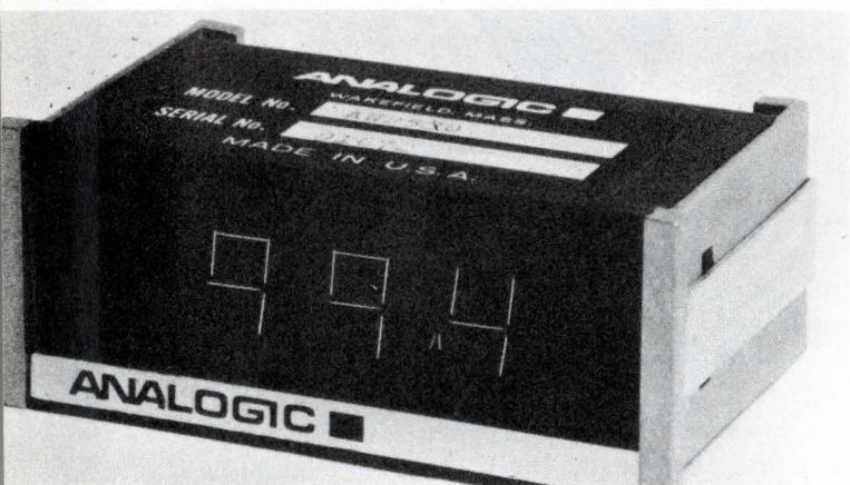
The 2530, from Analogic, is in the less than $50 class. It offers a 999 full scale reading and lets you program the display count so that you can scale the inputs, much like an analog meter.
