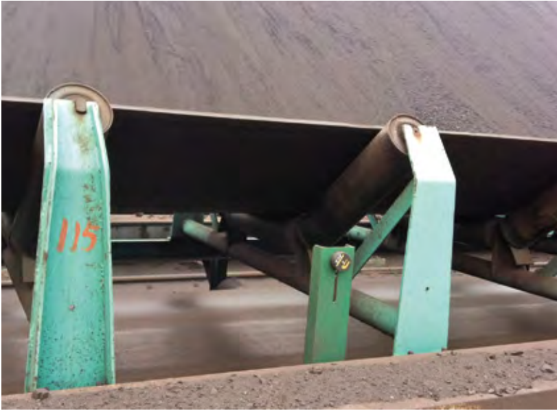
RFID data carriers are mounted on the conveyor belt of the bucket-wheel stacker reclaimer for position detection
