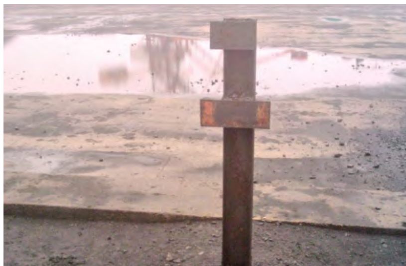
The solution previously used with metal flags for position control was too error-prone for the operators
