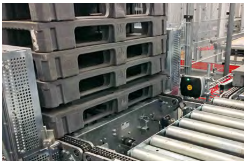
The plastic pallets come ex-factory with a UHF tag
