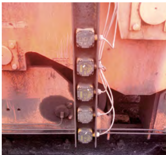
Four proximity sensors detect the metal flags for the code, the fifth triggers the recognition
