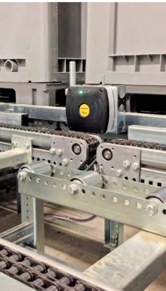
The LED indicates the status of the read/write head directly on the device
