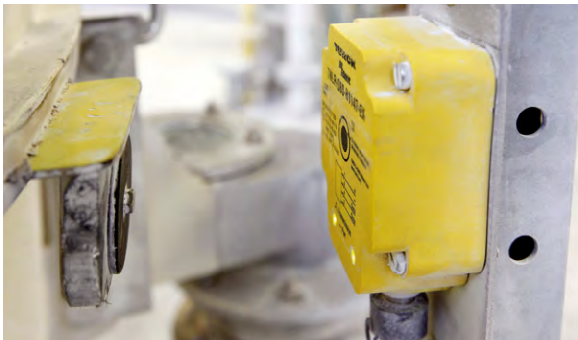
RFID is a robust medium to identify tools or, as shown here, impact screens
