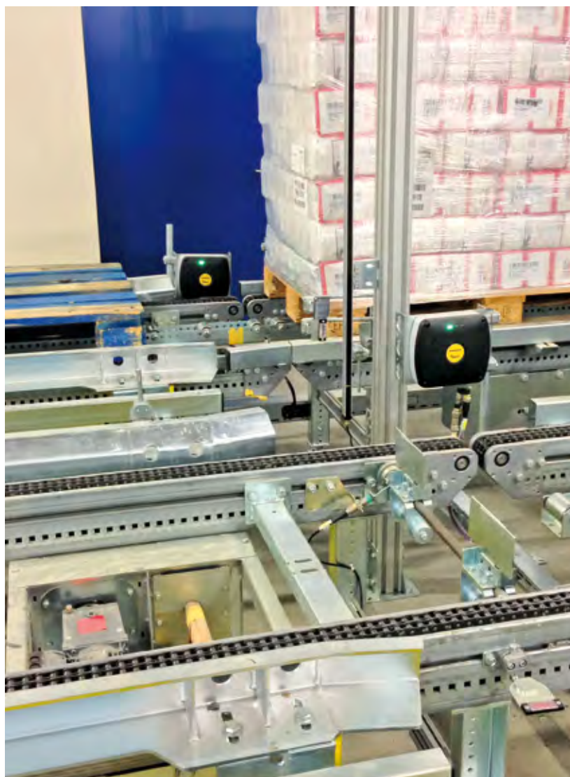
Neighbor conflicts excluded: Both read/write heads only read the pallets directly in front of them
