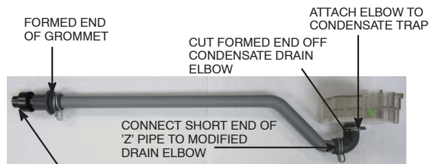
DRAIN ELBOW "Z" DISCHARGE PIPE FOR LEFT SIDE DRAIN IS ROUTED BEHIND INDUCER
