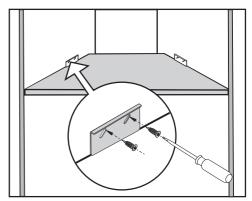
■ Secure the anti-tipping mechanism to the right and left-hand side walls of the housing unit with the 4 screws supplied (4 x 16 mm).
