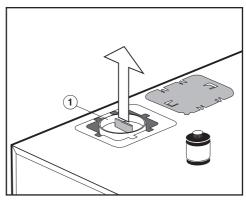
■ Pull the red transit device ① up and out, e.g. with universal pliers.
