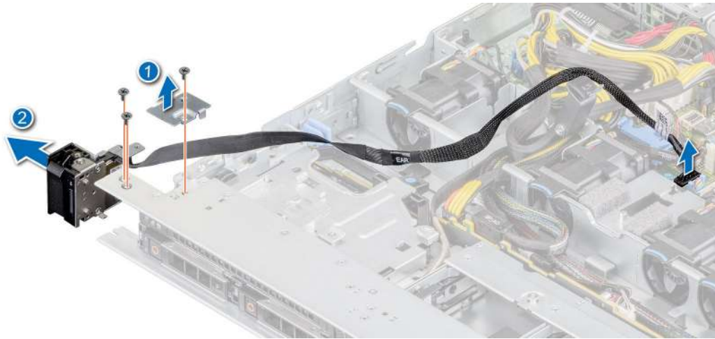
Figure 99. Removing the left control panel
