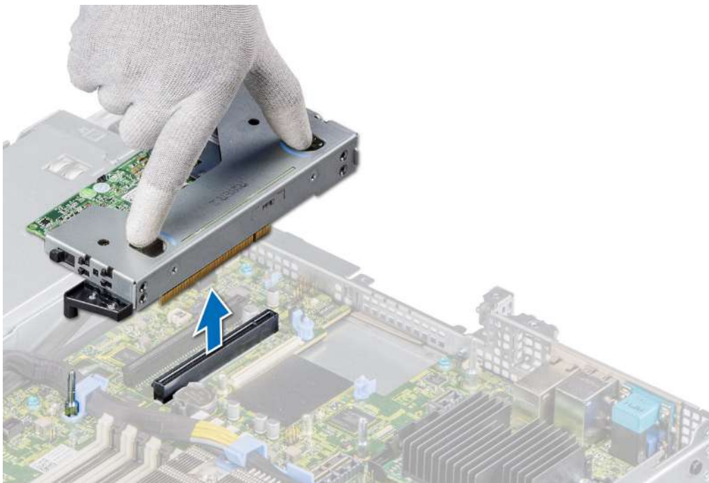
Figure 54. Removing the low profile left riser
