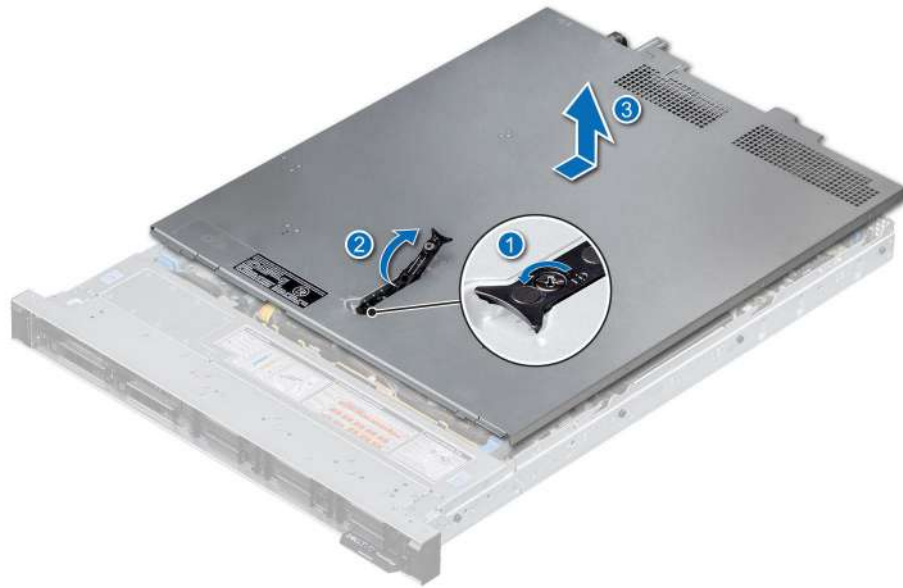
Figure 17. Removing the system cover
