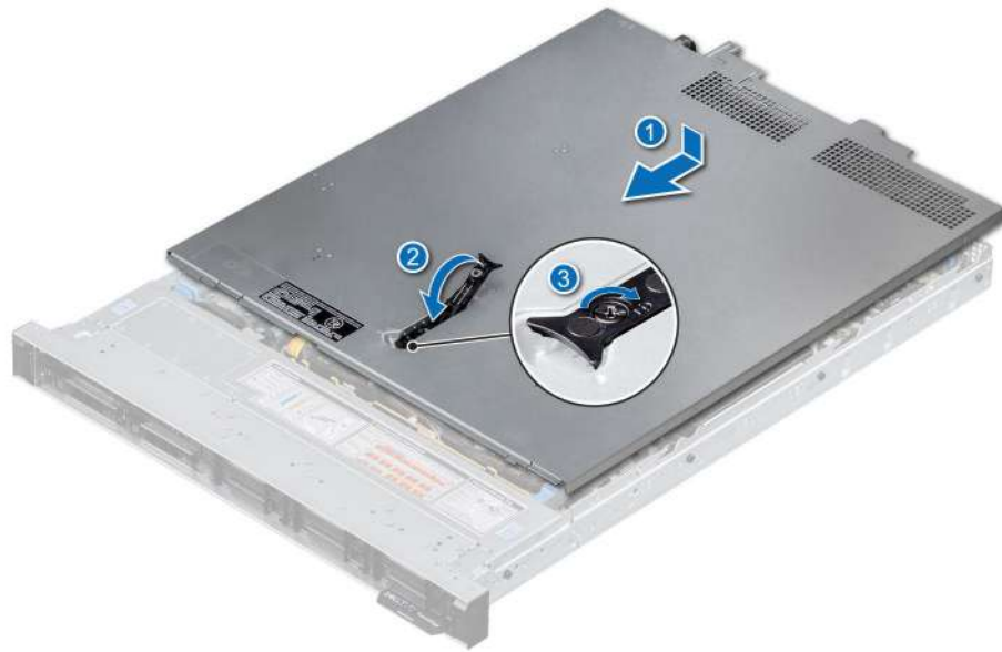
Figure 18. Installing the system cover
