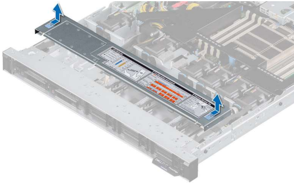
Figure 19. Removing the drive backplane cover
