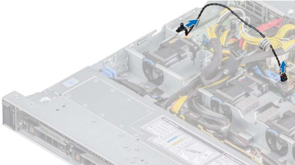
Figure 25. Removing the intrusion switch
