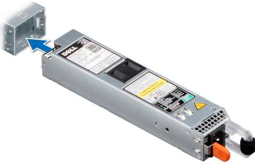
Figure 93. Installing a power supply unit
