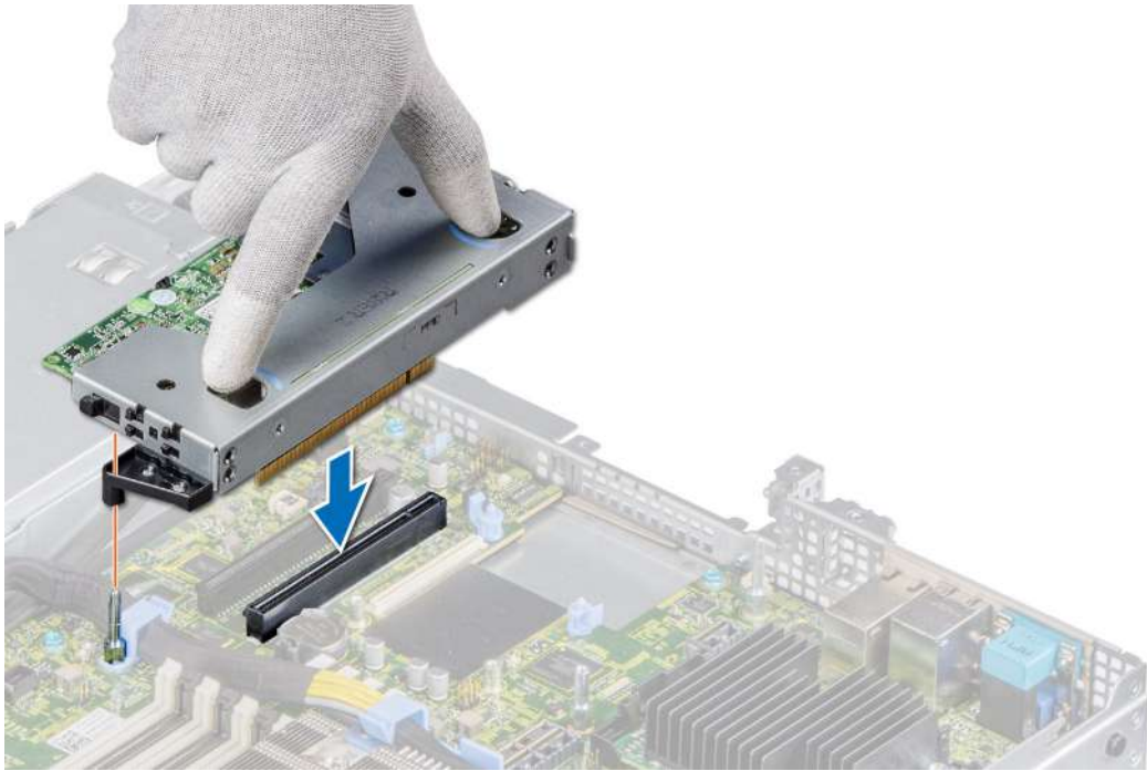
Figure 56. Installing the low profile left riser
