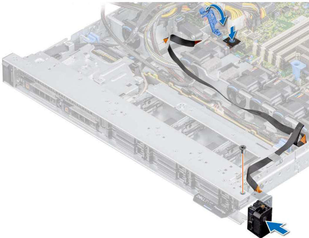
Figure 104. Installing the right control panel
