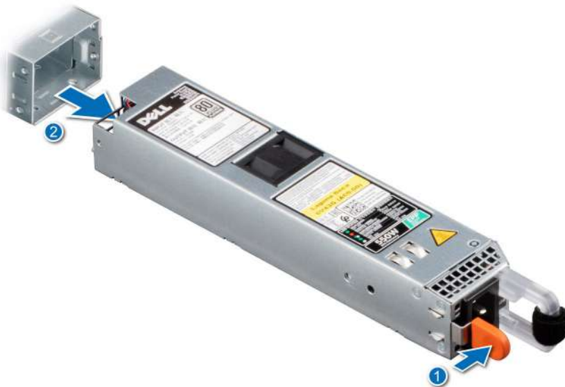
Figure 92. Removing a power supply unit
