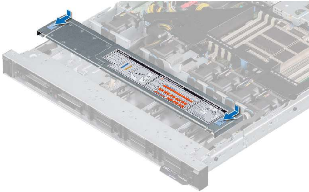
Figure 20. Installing the drive backplane cover
