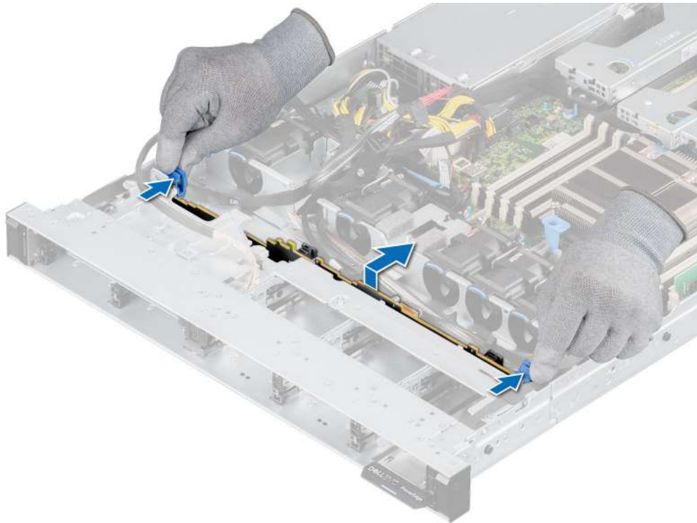
Figure 36. Removing the backplane
