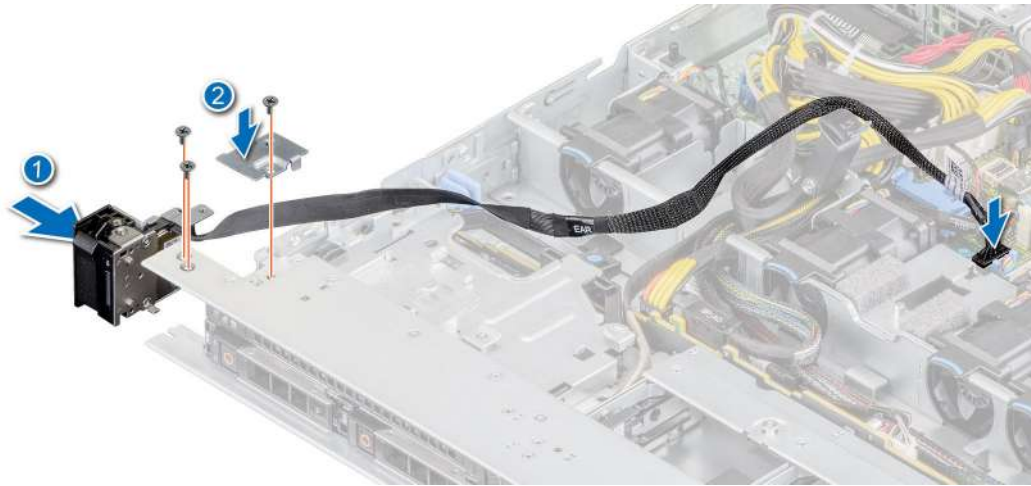
Figure 100. Installing the left control panel
