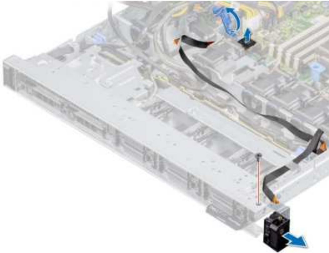
Figure 102. Removing the right control panel
