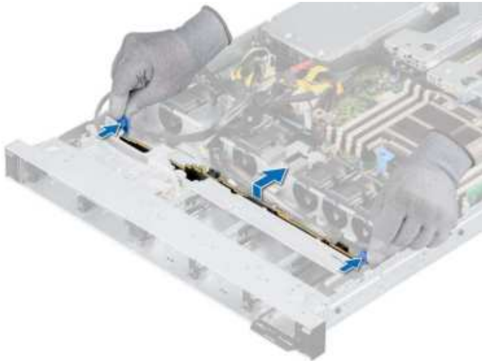
Figure 36. Removing the backplane
