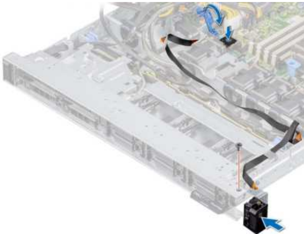
Figure 104. Installing the right control panel
