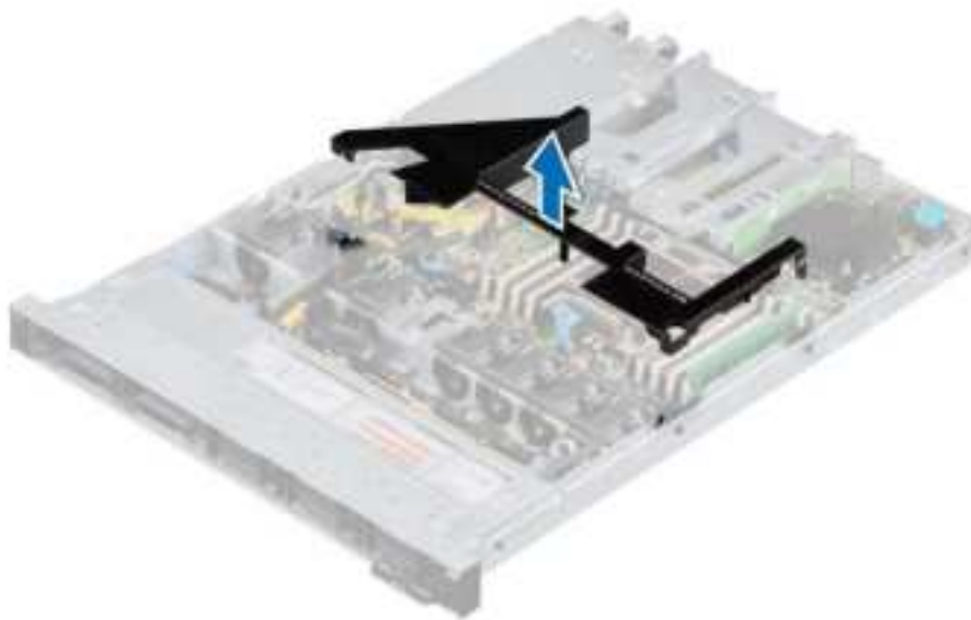
Figure 21. Removing the air shroud
