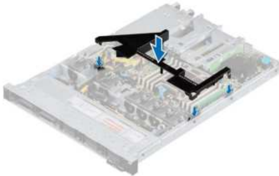
Figure 22. Installing the air shroud
