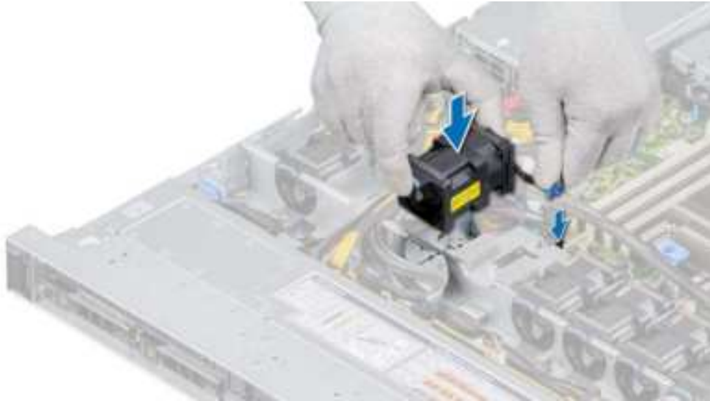
Figure 24. Installing a cooling fan
