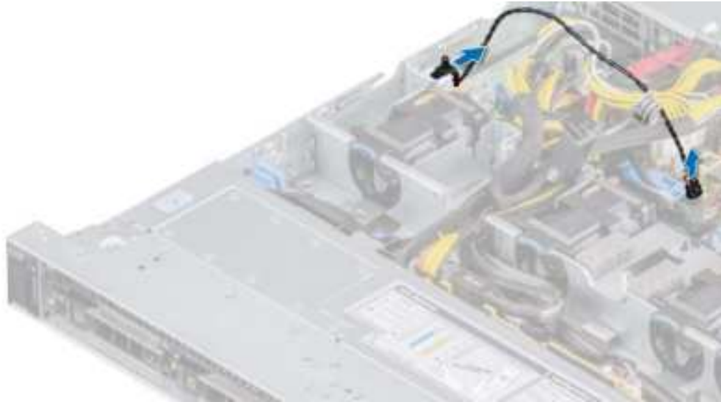
Figure 25. Removing the intrusion switch
