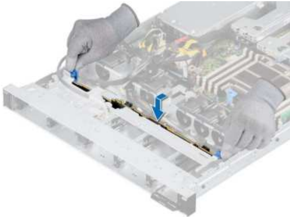
Figure 37. Installing the drive backplane
