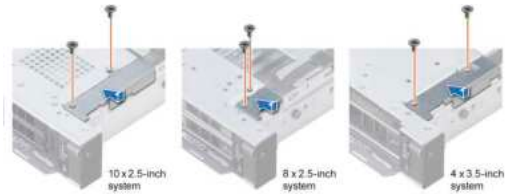
Figure 103. Installing the cable cover
