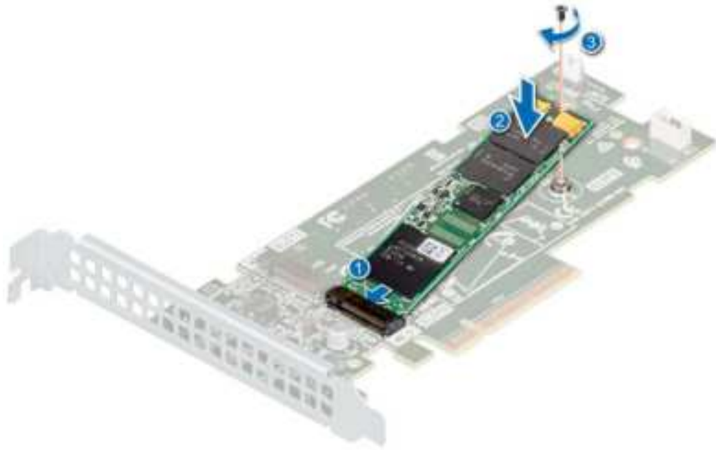
Figure 69. Installing the M.2 SSD module
