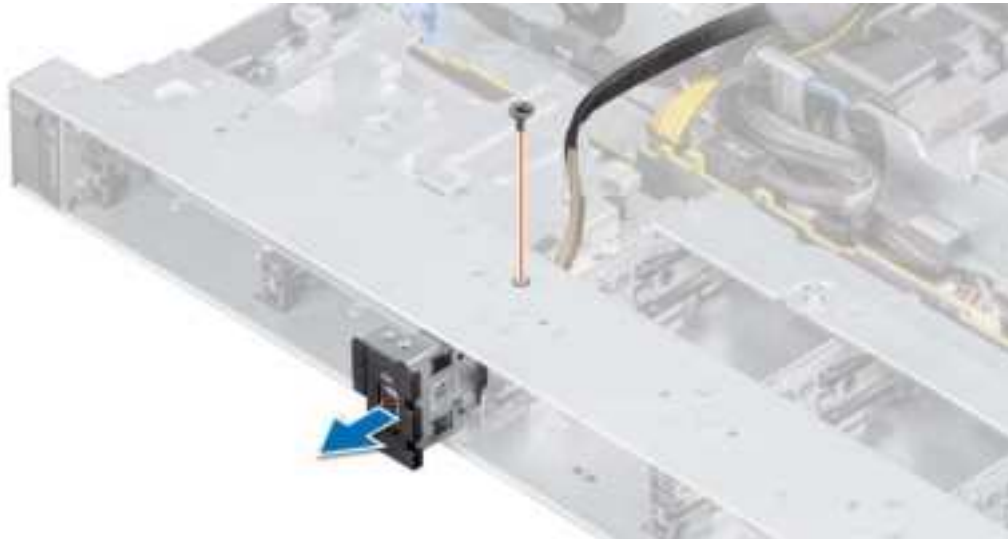
Figure 86. Removing the VGA module
