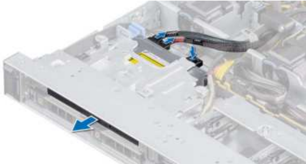
Figure 88. Removing the optical drive
