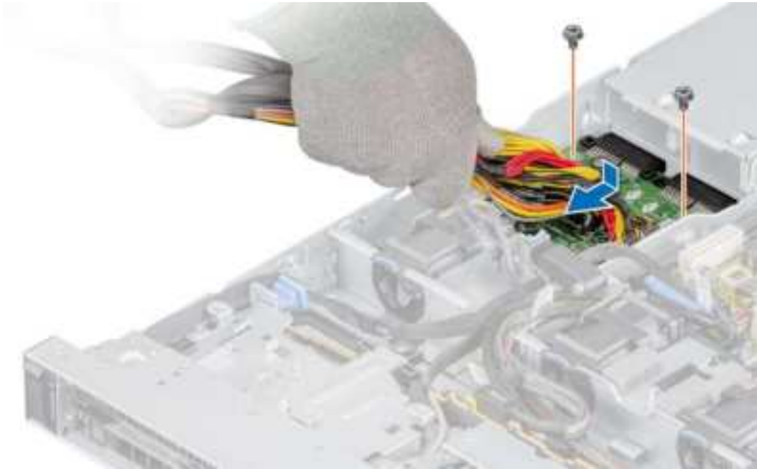
Figure 95. Installing the power interposer board
