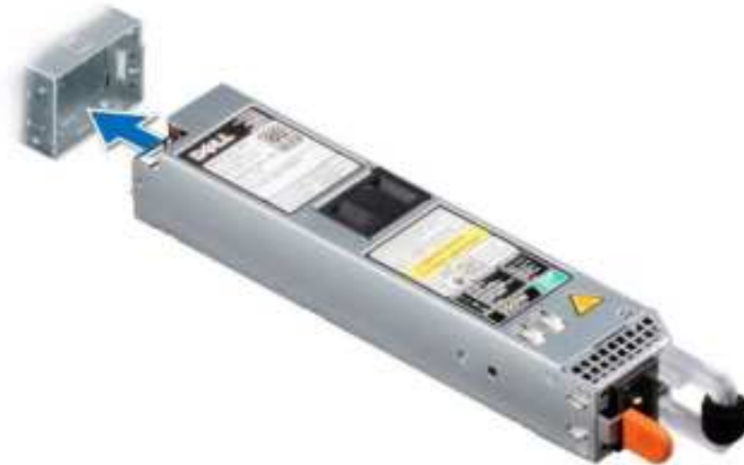
Figure 93. Installing a power supply unit
