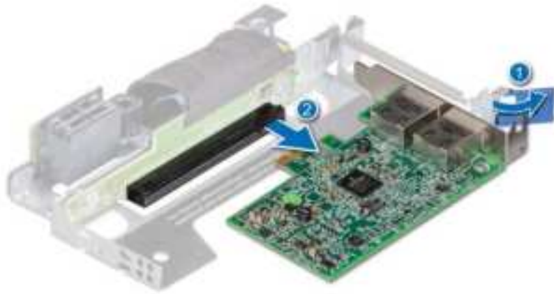
Figure 59. Removing an expansion card from the low profile right riser
