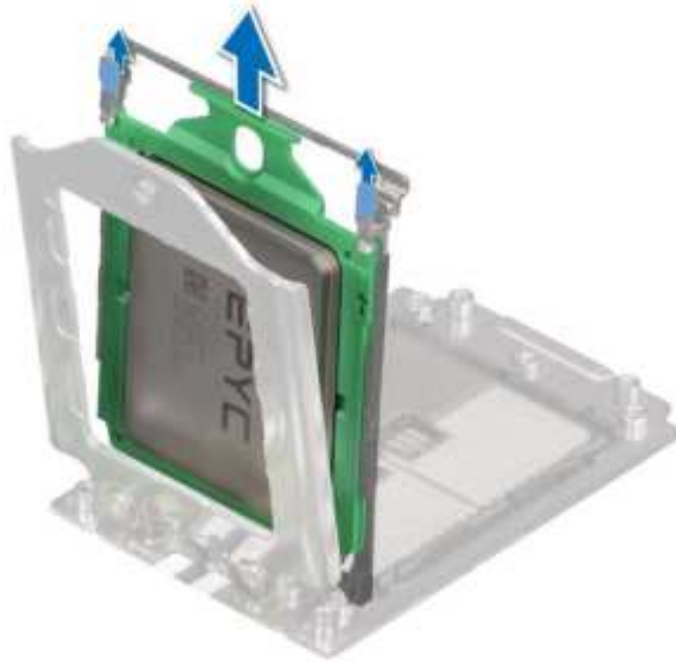
Figure 48. Removing the processor tray
