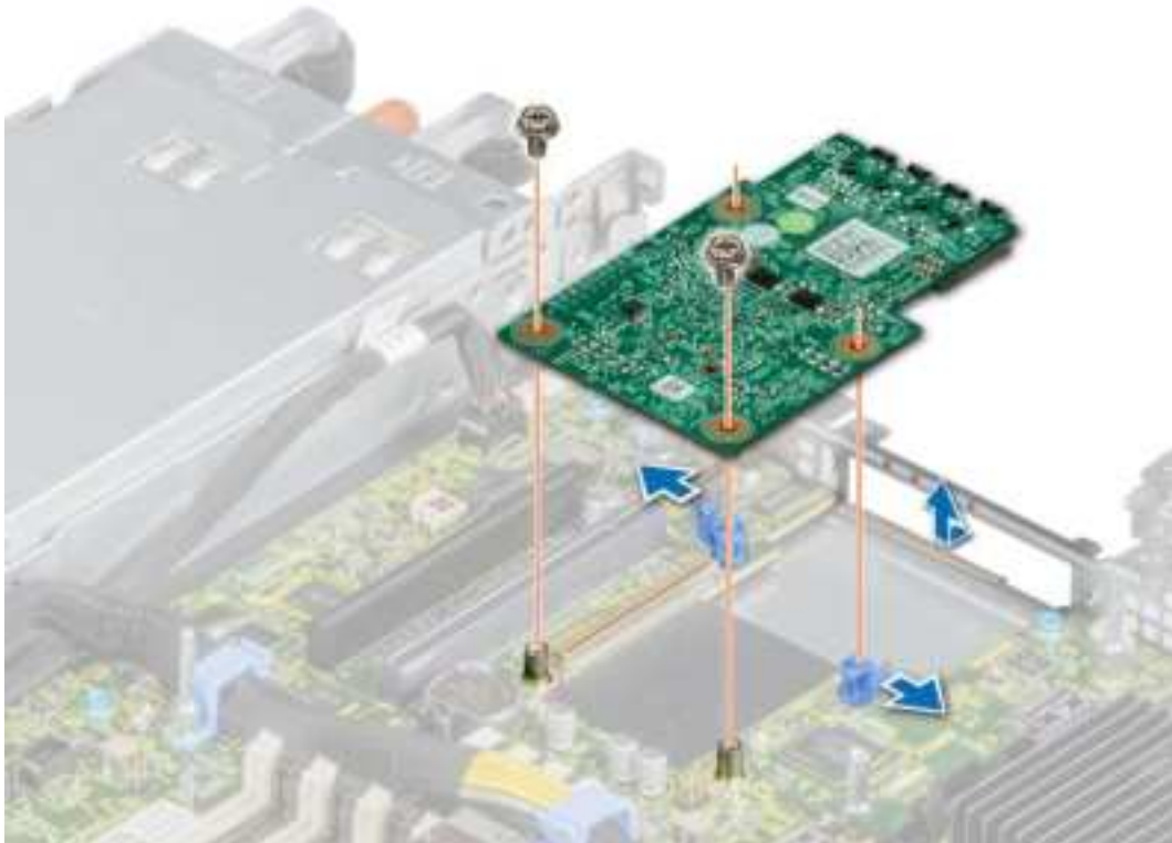
Figure 72. Removing the LOM riser card
