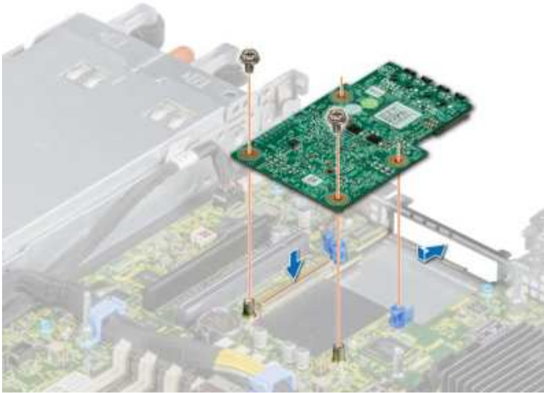
Figure 77. Installing the LOM riser card
