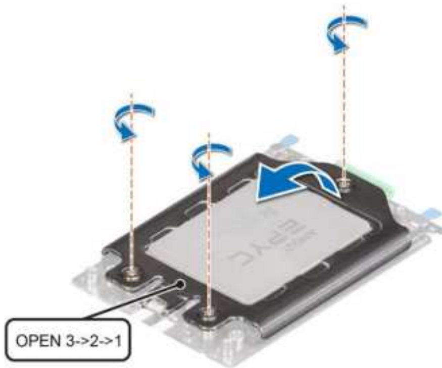
Figure 46. Removing screws on the force plate
