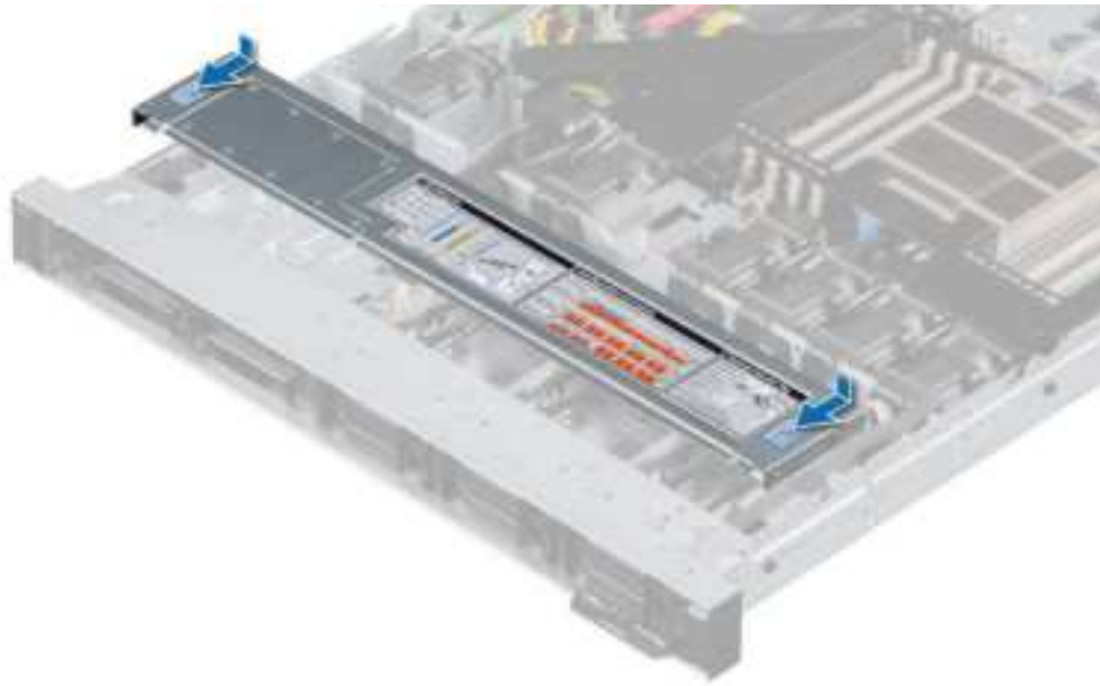
Figure 20. Installing the drive backplane cover
