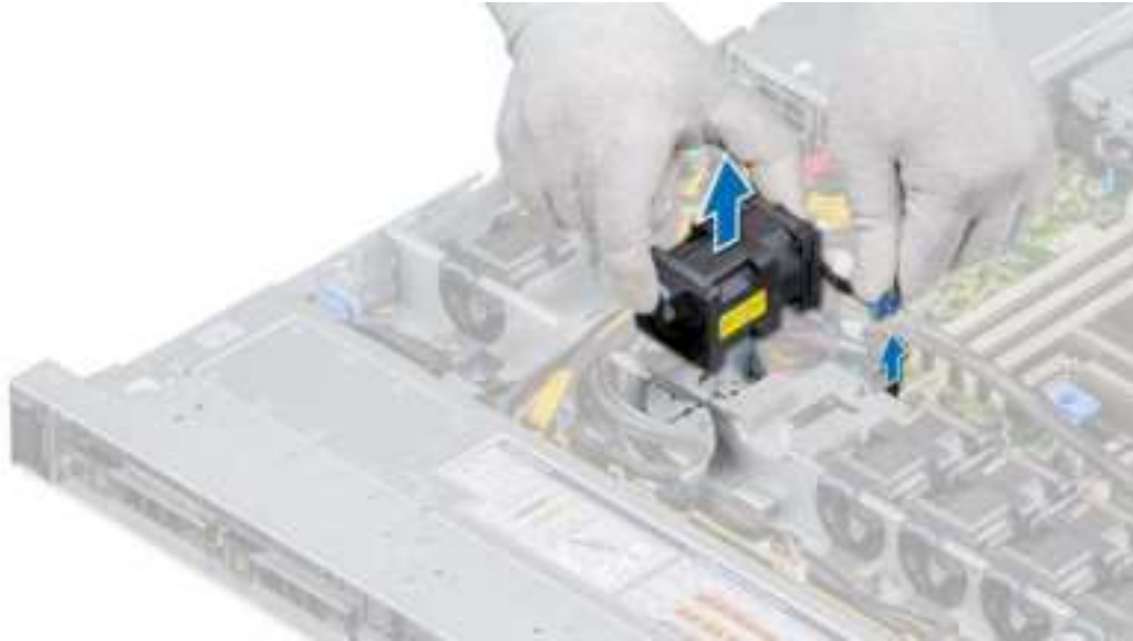
Figure 23. Removing a cooling fan
