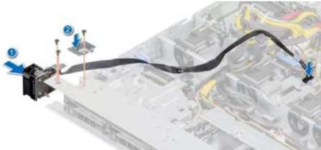
Figure 100. Installing the left control panel
