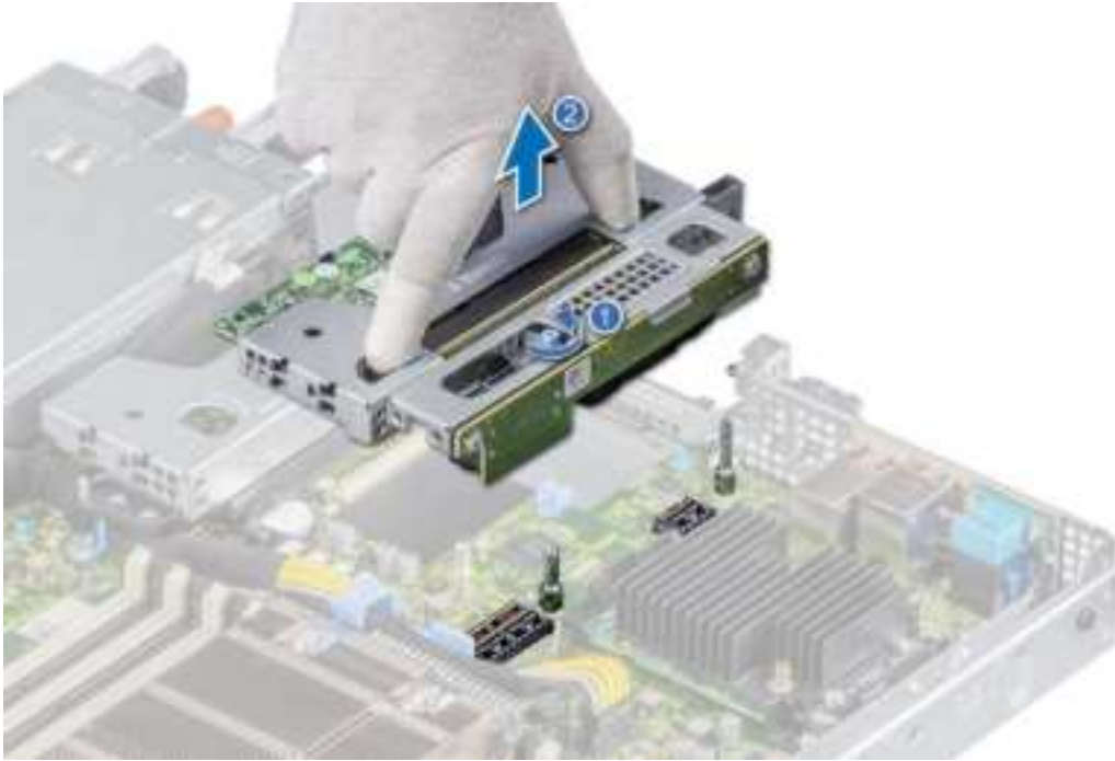
Figure 55. Removing the low profile right riser
