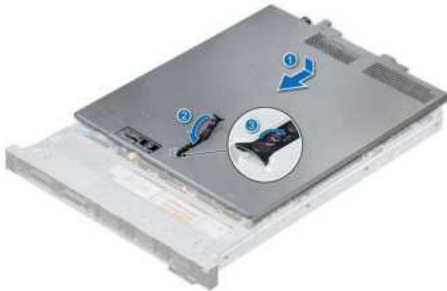
Figure 18. Installing the system cover
