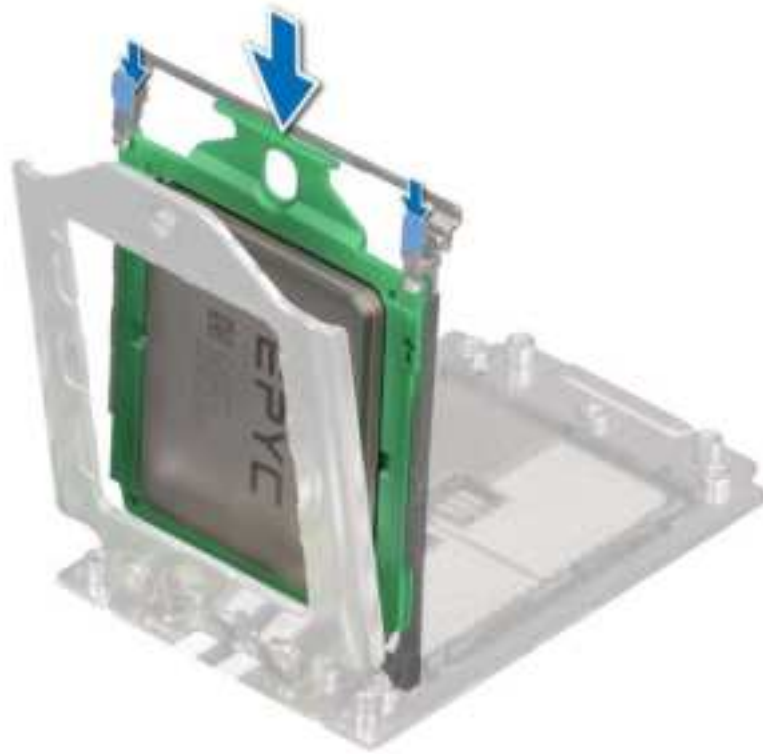
Figure 49. Placing the processor tray into the rail frame
