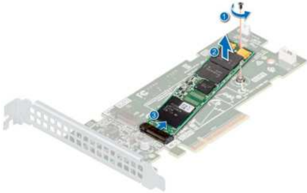
Figure 68. Removing the M.2 SSD module
