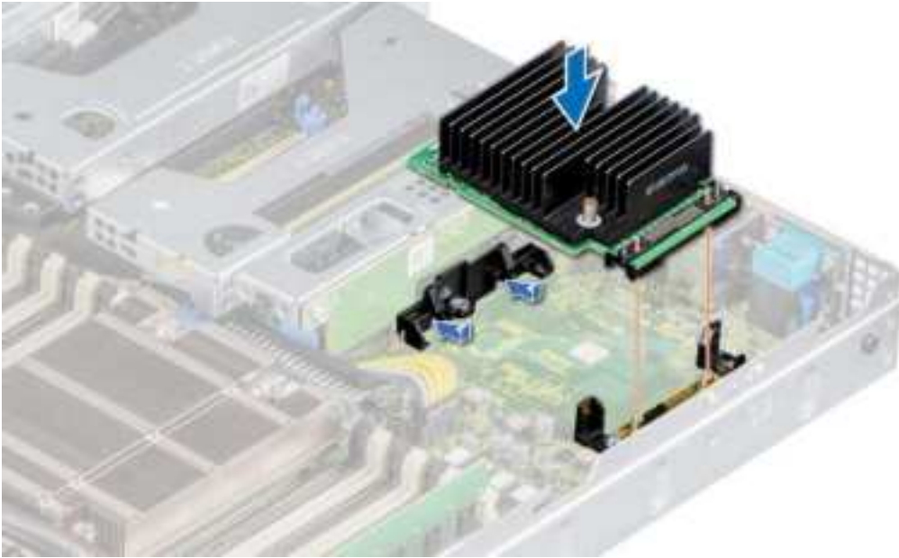
Figure 80. Installing the mini PERC card
