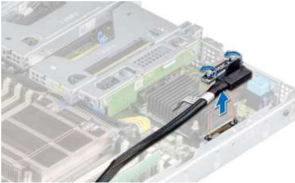
Figure 78. Removing the mini PERC card cable
