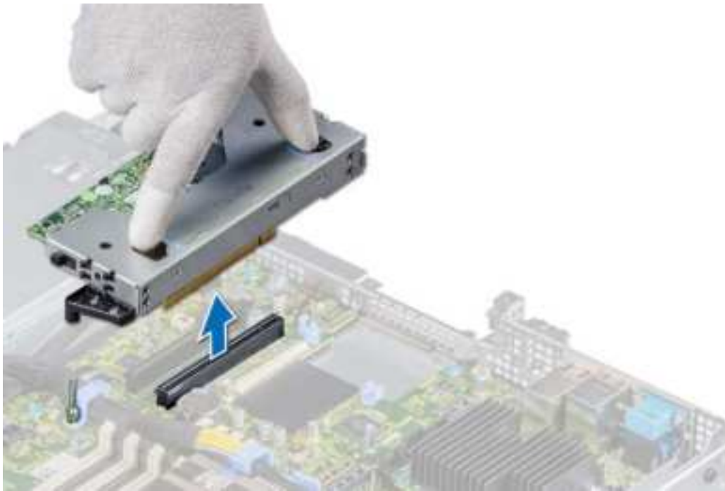
Figure 54. Removing the low profile left riser
