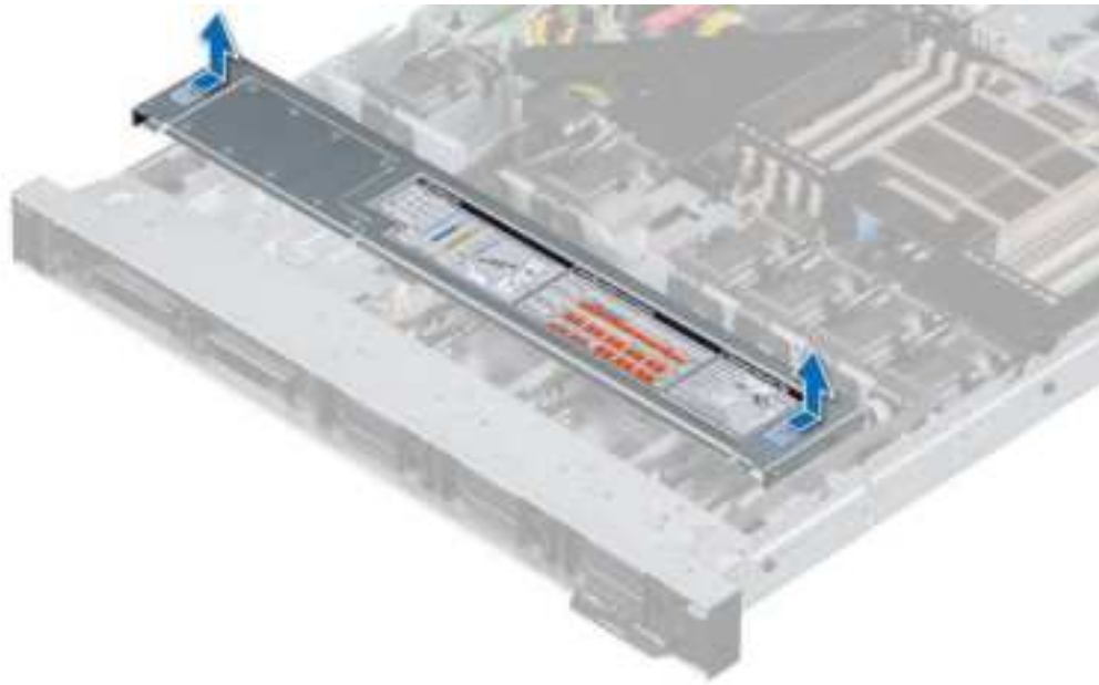
Figure 19. Removing the drive backplane cover
