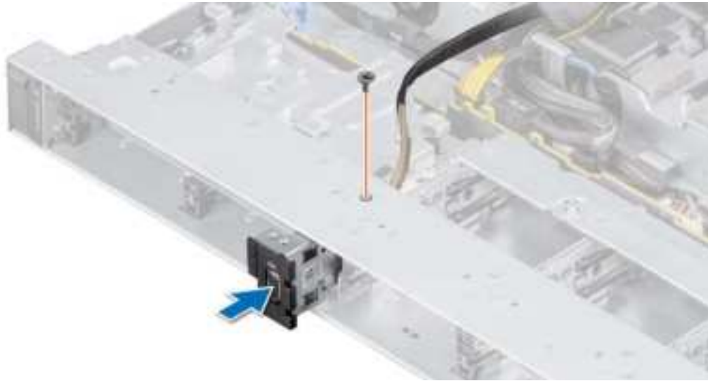
Figure 87. Installing the VGA module
