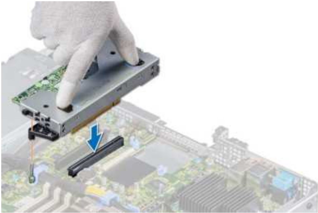
Figure 56. Installing the low profile left riser
