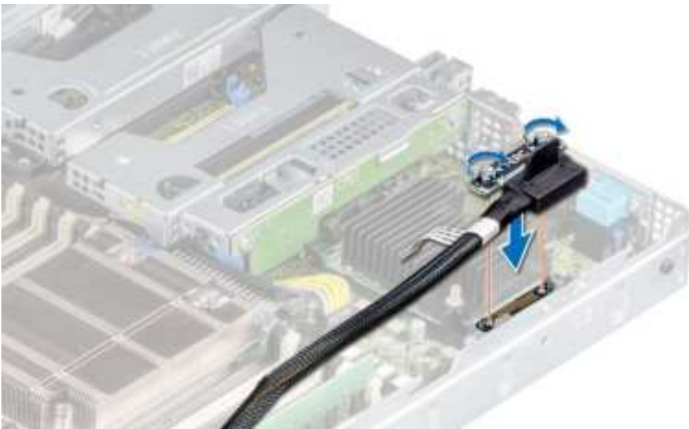
Figure 81. Installing the mini PERC card cable
