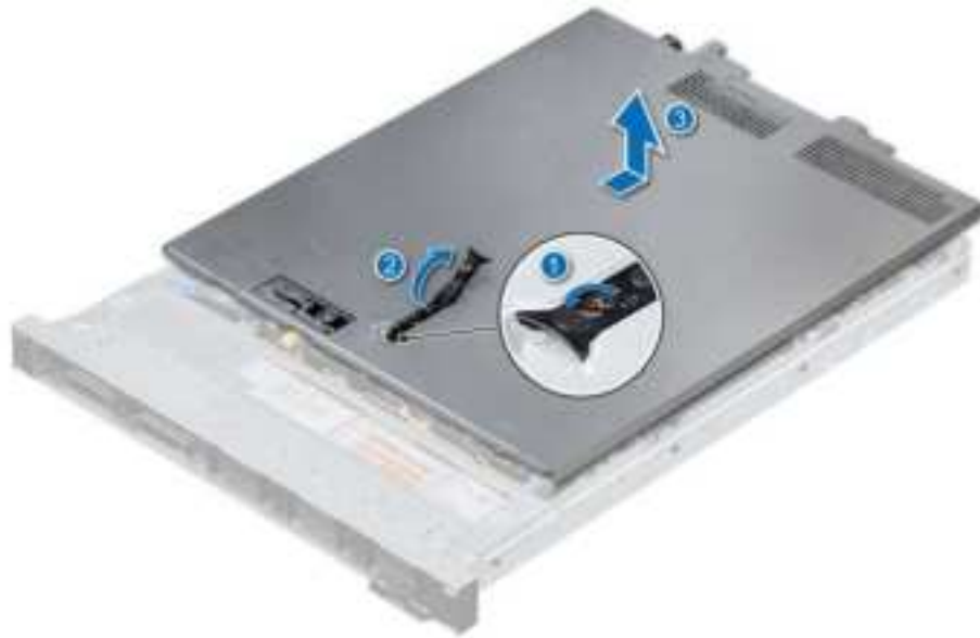
Figure 17. Removing the system cover
