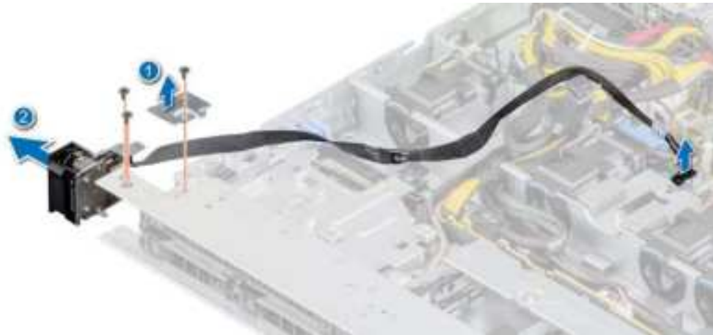
Figure 99. Removing the left control panel
