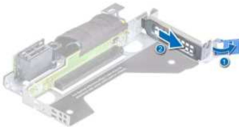
Figure 63. Removing a filler bracket from a low profile right riser
