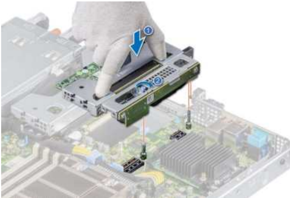
Figure 57. Installing the low profile right riser
