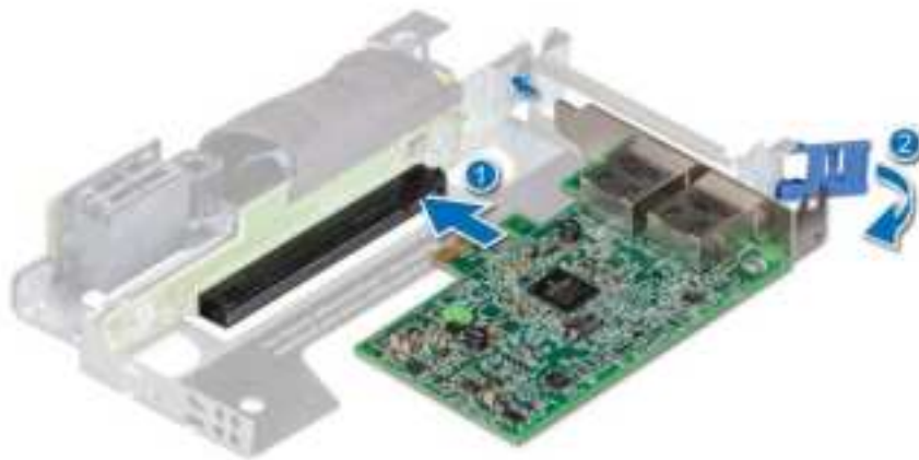
Figure 65. Installing an expansion card into a low profile right riser
