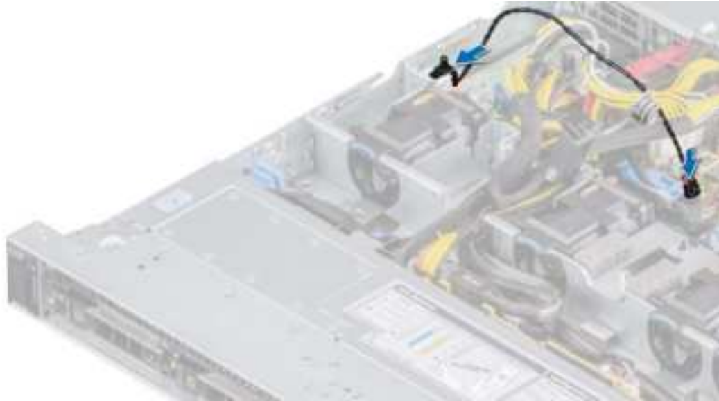
Figure 26. Installing the intrusion switch
