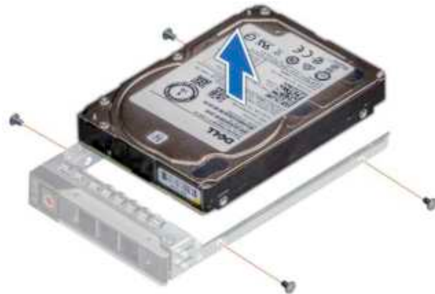
Figure 31. Removing the drive from the drive carrier
