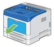
4 Grasp both sides of the bypass tray, and then pull the bypass tray from the printer.
