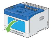
2 Grasp both sides of the bypass tray, and then pull the bypass tray from the printer.
