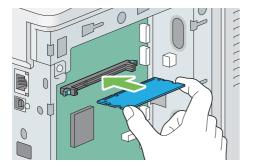
5 Push the memory module firmly into the slot.
