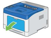
3 Grasp both sides of the bypass tray, and then pull the bypass tray from the printer.
