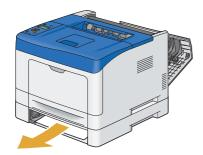
5 Insert the optional 250 sheet feeder into the printer, and push until it stops.
