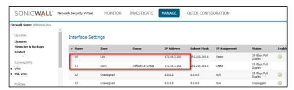
7 Add secondary firewall HA interface. Navigate to Home > Virtual Machines page and select the secondary virtual machine that you have created during deployment. On the left panel, select Settings > Networking, configure NIC Private IP of X2 as shown below.
