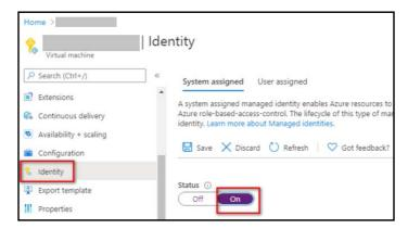
3 Enable Identity of Secondary Virtual Machine. To enable, navigate to **Home > Virtual Machines** page, search for the secondary virtual machine that you have created during deployment and on the left panel, select **Identity** and change the status to **On**.
