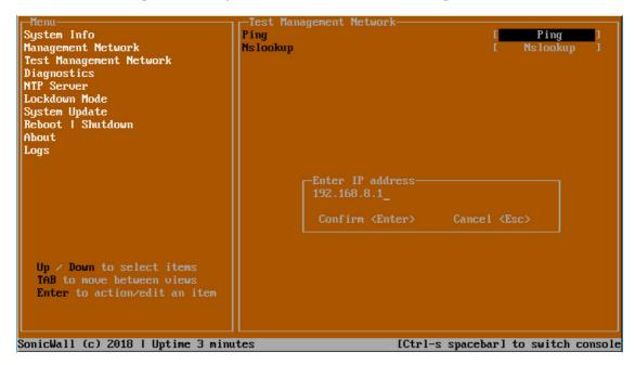
The **Test Management Network** screen provides the **Ping** and **Nslookup** tools to test connectivity between the management interface and the local network. **Ping** is used to test whether hosts in the network are reachable. **Nslookup** is available for sending DNS queries from the NSv appliance.
