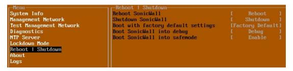
The **Reboot | Shutdown** screen provides functions for rebooting the NSv appliance, enabling debug mode, and enabling SafeMode. To perform an action, position the focus and then press **Enter** to select the desired action. Select **Yes** in the confirmation dialog, then press **Enter** again.
