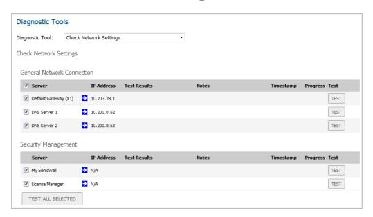
**Check Network Settings** is a diagnostic tool that automatically checks the network connectivity and service availability of several pre-defined functional areas of the NSv Series, returns the results, and attempts to describe the causes if any exceptions are detected. This tool helps you locate the problem area when users encounter a network problem.
