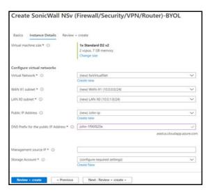
6 Select **Virtual machine size**, then select the row with the Azure equivalent for the NS*v* model you want to deploy in the **Choose a size** screen. Click **Select**.
