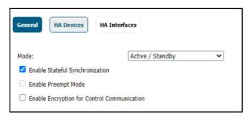
11 Click **HA Devices** tab and enter the serial number from the secondary. You can find the serial number in the **Monitor > System Status** page.
