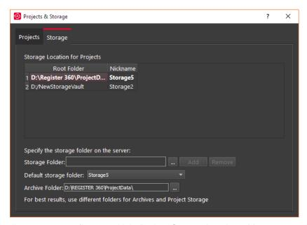
The Storage tab allows you to configure multiple Project Storage locations. You can use this feature to create and toggle between datasets on multiple drives. For best results, use internal SSD drives and create separate folders for Storage and Archive.
