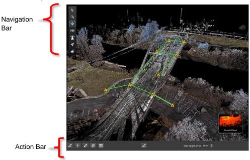
7.8. At any point, the user may access their "Settings" by clicking on the gear icon at the very top left of the screen to change units and set the error threshold for green, yellow and red links.
