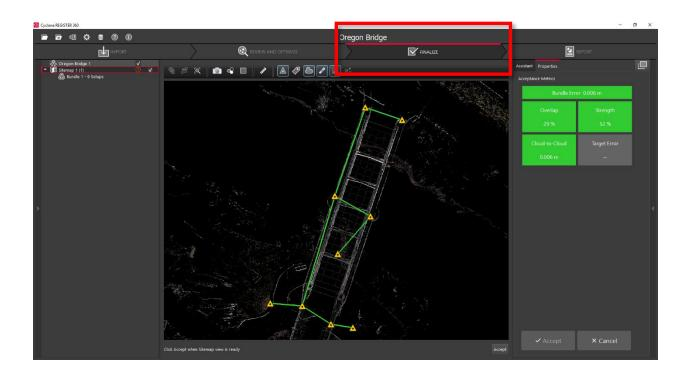
8.1. Within the "Finalize" stage the user can make final adjustments to the presentation of their project by turning On or Off the point cloud, setups, links, sitemap, and setup labels.
