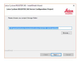
NOTE! The storage folder for Cyclone REGISTER 360 should NOT be the same folder as the JetStream Storage folder if JetStream is installed on the same computer.
