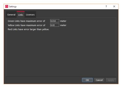
The Links tab allows you to customize your error thresholds for Links. You can adjust what levels of error will be represented by your green/yellow/red link lines. By default, these will be set to 0.015 and 0.02 m respectively.
