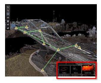
7.6.1.The user should use the "TruSlicer" view to QA their regsiration. The point clouds from each setup will be colored differently. A good alignment will show a thorough intermixing of colored points and matching geometry in areas of overlap. The user can control the thickness and location of the slice via the sliders at the top left of the workspace.
