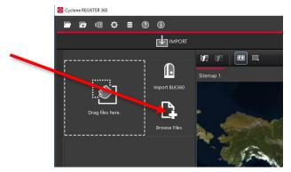
3.5. "Import BLK360" will launch a new Cyclone REGISTER 360 window that will allow you to connect to a local BLK360 Imaging Scanner and select individual files to import.
