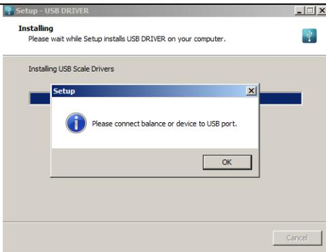
Connect the scale to a computer, use 1.8-meter long USB A/B cable maximum (in case of already connected scale, it is necessary to disconnect it and reconnect using USB cable). Respective message box is displayed, press **OK** button for confirmation.
