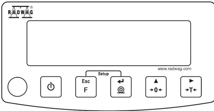
Figure 5. Operation panel of WTC series scales
