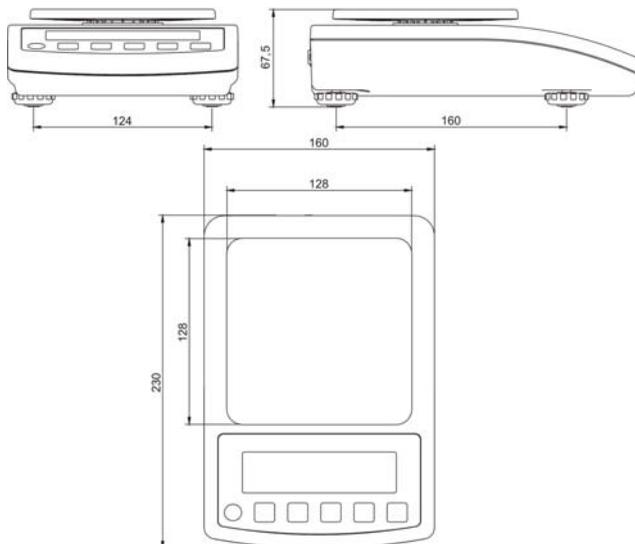
Figure 2. Dimensions of WTC 600, WTC 2000, WTC 3000 scale
