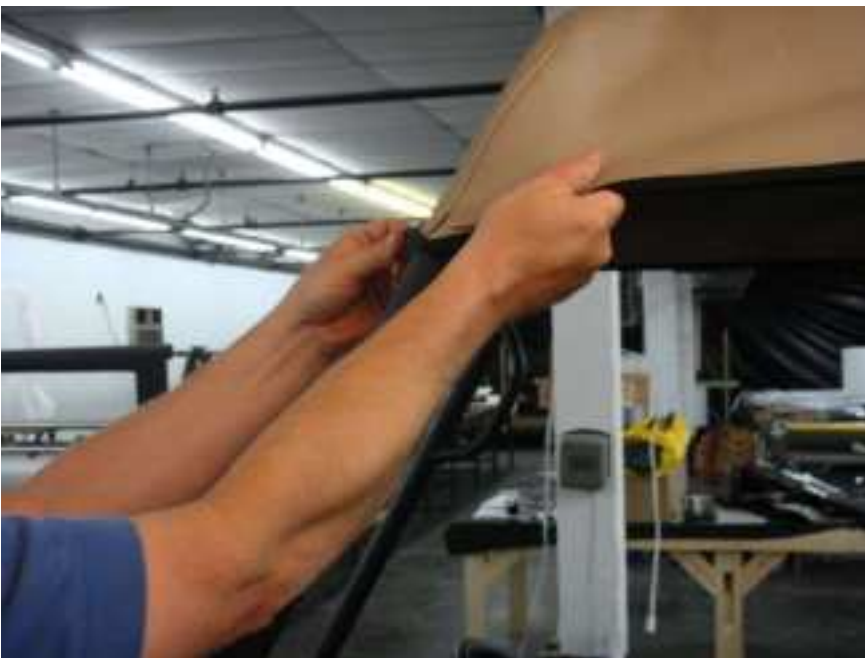
Figure 4.1 - Attach front and rear Enclosure Velcro tabs to installed Velcro strips
