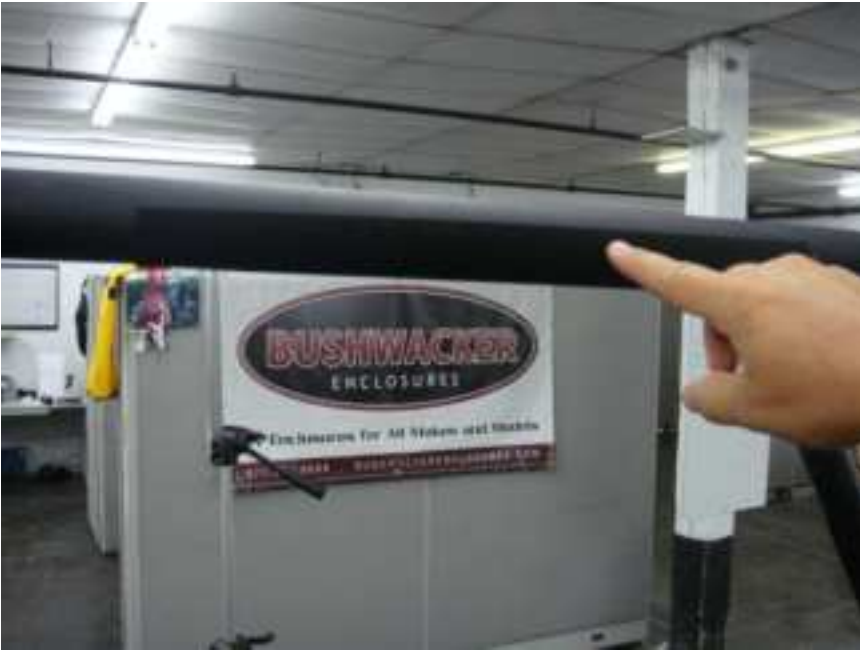
Figure 3.1 – adhere 13” Velcro strips above the door area on the Roll Bar Cross-member
