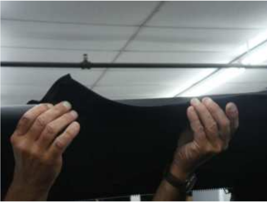
Figure 4.2 – attach Top Cap top side roll bar tabs to installed 13” Velcro strips
