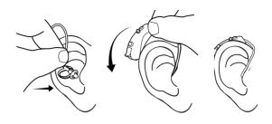
The illustrations show an open ear-tip. For further information on ear-tip/earmould types, anchors and procedures, see the separate ear-set user manual provided.
