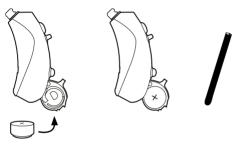
If the battery drawer does not close easily, the battery is incorrectly inserted.
