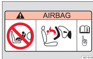
Fig. 20 Passenger's side sun visor: airbag sticker.
