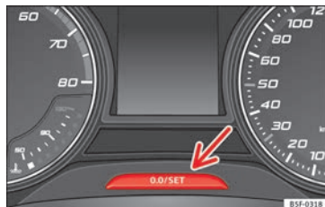
Fig. 106 Instrument panel: odometer and reset button.
