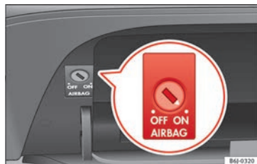
Fig. 78 In the glove compartment: Switch for activating and deactivating the front passenger airbag
