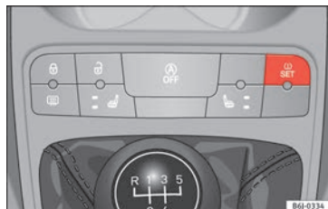
Fig. 159 Centre console: tyre monitoring system button.
