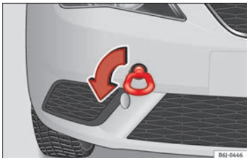
Fig. 81 Towline anchorage at the front of the vehicle
