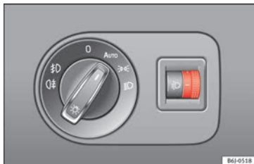
Fig. 119 Dash panel: headlight range control.
