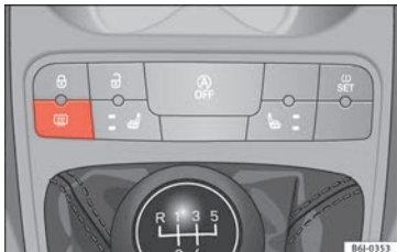
Fig. 120 Centre console: heated rear window switch.
