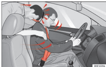
Fig. 75 The unbelted passenger in the rear seat is thrown forward violently, hitting the driver who is wearing a seat belt.
