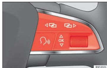
Fig. 35 Right side of multifunction steering wheel: control buttons.
