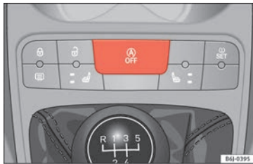
Fig. 148 The Start-Stop function button.
