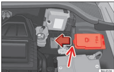
Fig. 52 In the engine compartment: fuse box cover.
