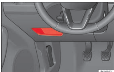
Fig. 51 On the driver-side dash panel: fuse box cover.
