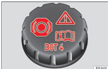
Fig. 49 Engine compartment: brake fluid reservoir cap.
