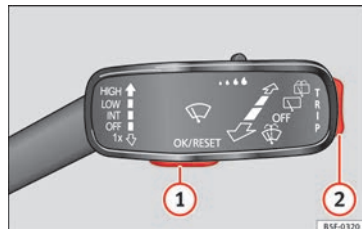
Fig. 34 Windscreen wiper lever: control buttons.
