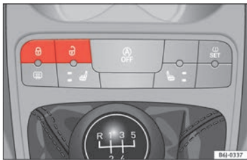
Fig. 2 Centre console: Central lock buttons.
