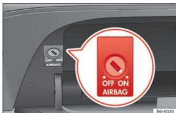
Fig. 16 Front passenger front airbag switch.
