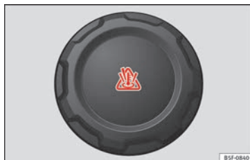
Fig. 48 Engine compartment: coolant expansion tank cap.
