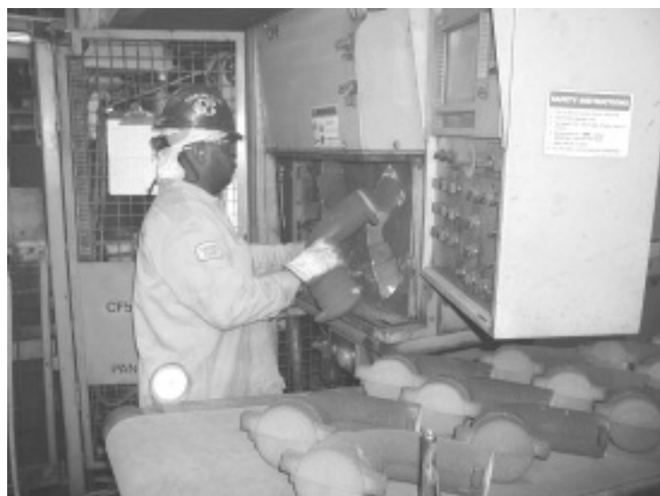
Figure 13—Automatic Core Setter.
