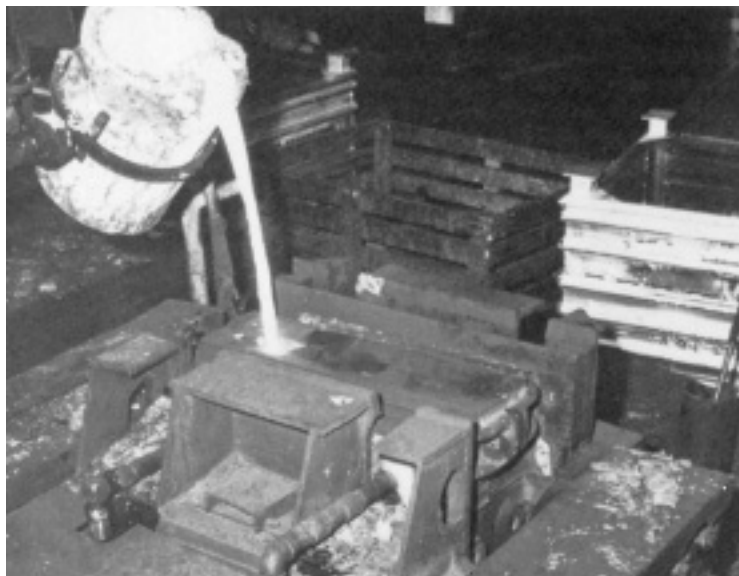
Figure 18—Permanent-Mold Casting for Fittings Production.
