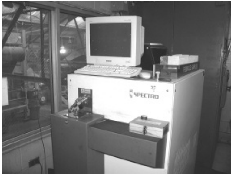
Figure 23—Optical Emission Spectrometer (OES): Analysis of Irons, Production Control Samples, and Final Product.
