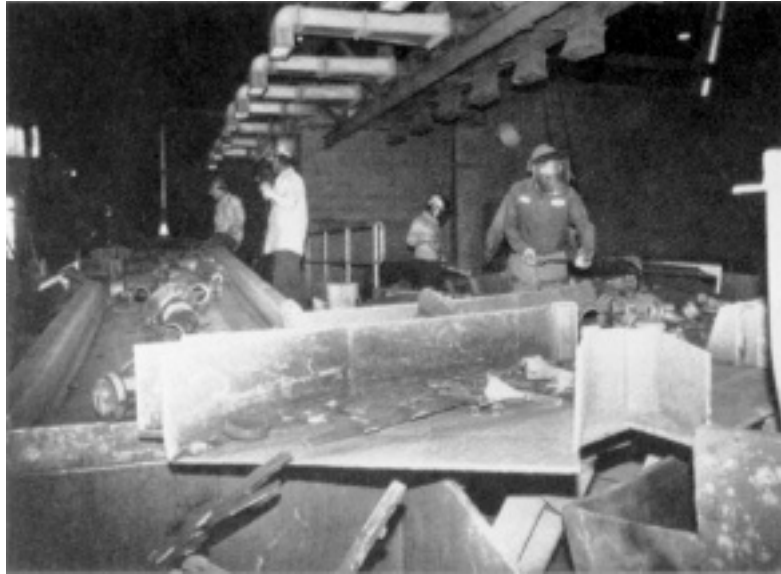
Figure 16—Castings Being Shaken Out of the Mold.
