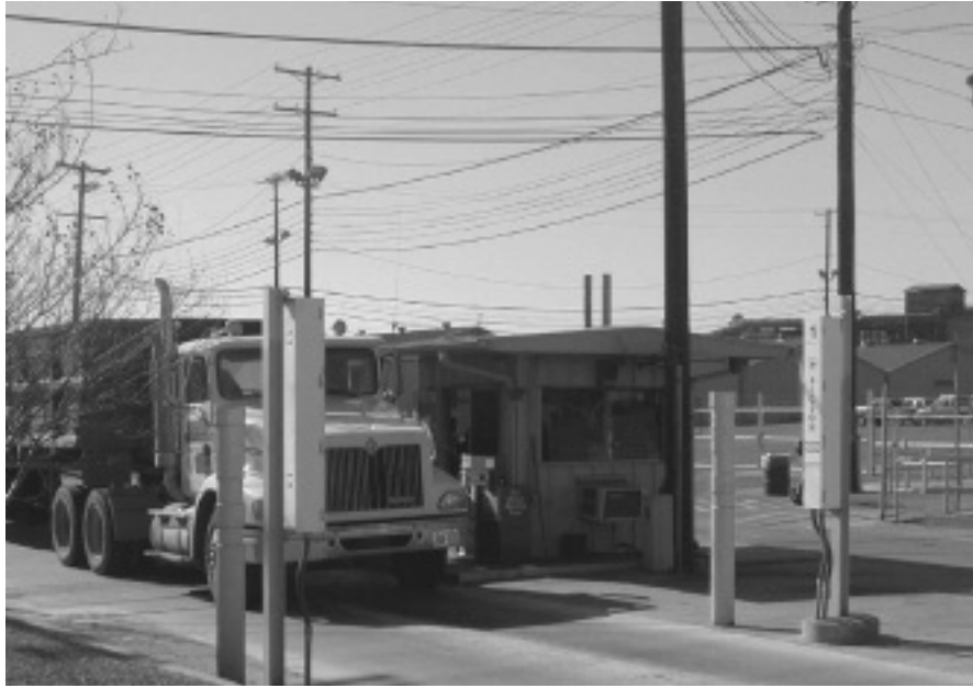
Figure 1—Radiation Detector Screening Ferrous New Material for Radiation.
