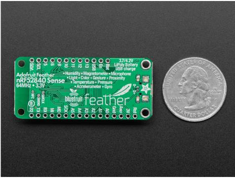
A chorus of supporting sensors surround the module so you can do all sorts of **environmental and motion sensing**:
