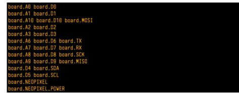
Each line represents a single pin. Find the line containing the pin name that's labeled on the physical board, and you'll find the other names available for that pin. For example, the first pin on the board is labeled **A0**. The first line in the output is board.A0 board.D0. This means that you can access pin **A0** with both board.A0 and board.D0.
