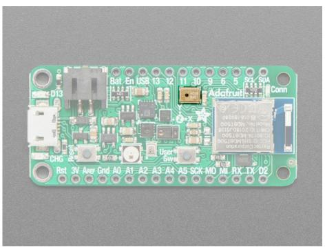
**PDM Microphone sound sensor: MP34DT01-M** - PDM sound sensor. In CircuitPython, **board.MICROPHONE\_DATA** is PDM data, and **board.MICROPHONE\_CLOCK** is PDM clock. In Arduino, **D34** is PDM data, and **D35** is PDM clock.
