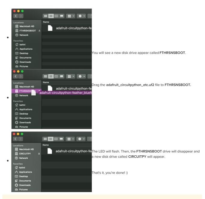
Note: Some early release Sense boards had the drive named FTHR840BOOT. You can still copy .UF2s to the board, just copy to the board name appearing when the board is plugged in.
