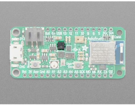
**Gyro + Accel: LSM6DS33** - This sensor is a 6-DoF IMU accelerometer + gyroscope. The 3-axis accelerometer, can tell you which direction is down towards the Earth (by measuring gravity) or how fast the Feather Sense is
