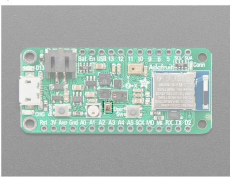
**Temp + Pressure: BMP280** - This sensor is a precision sensing solution for measuring barometric pressure with  $\pm 1$  hPa absolute accuracy, and temperature with  $\pm 1.0^{\circ}$ C accuracy. Because pressure changes with altitude, and the pressure measurements are so good, you can also use it as an altimeter with  $\pm 1$  meter accuracy. It has a low
