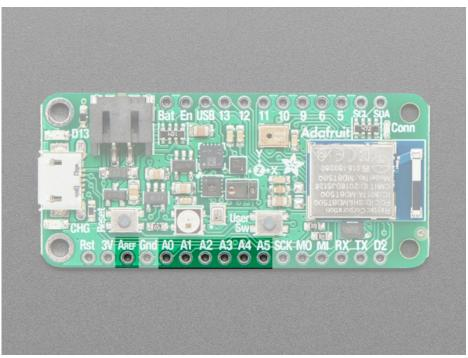
The **6** available analog inputs (**A0** .. **A5**) can be configured to generate 8, 10 or 12-bit data (or 14-bits with oversampling), at speeds up to 200kHz (depending on the bit-width of the values generated), based on either an internal 0.6V reference or the external supply.
