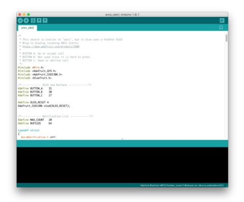
Make sure that the Adafruit\_SSD1306.h file has the 'SSD1306\_128\_32' macro enabled. Running the sketch with 'SSD1306\_128\_64' set will cause corrupted data to appear on the OLED display.
