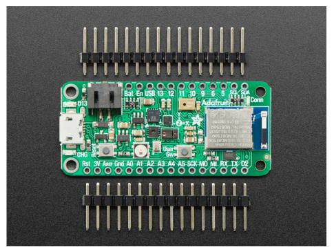
This Feather is also a **BLE-friendly CircuitPython board**! CircuitPython works best with disk drive access, and this is the only BLE-plus-USB-native chip that has the memory to handle running a little Python interpreter. The massive RAM and speedy Cortex M4F chip make this a good match. Make BLE central or peripheral devices with the ease of CircuitPython.
