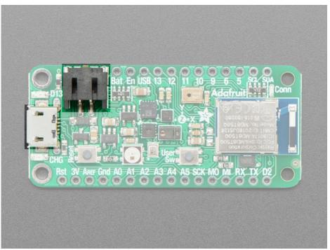
The above shows the Micro USB jack (left), Lipoly JST jack (top left), as well as the changeover diode (just to the right of the JST jack) and the Lipoly charging circuitry (to the right of the JST jack). There's also a **CHG** LED, which will light up while the battery is charging. This LED might also flicker if the battery is not connected.
