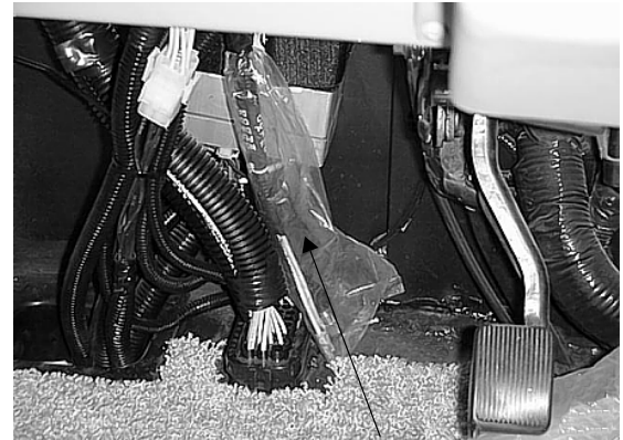
CB Wires (in plastic sheath)
