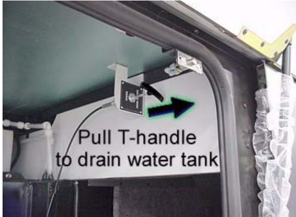
Water Tank Drain Valve (pull to open)
