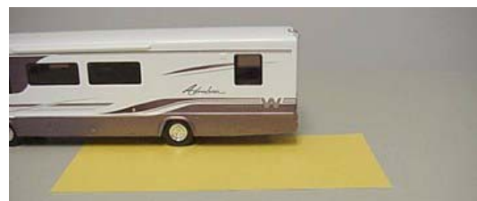
Weighing Left Rear 'Corner'
