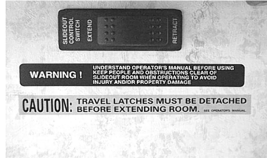
Rear Slideout Switch (on wall in rear of couch - varies by model)
