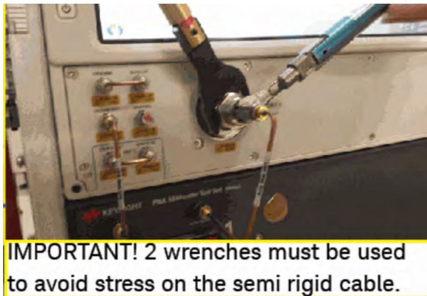
Figure 3-8 To avoid damaging your RF ports 1/2/3/4, always use two wrenches
