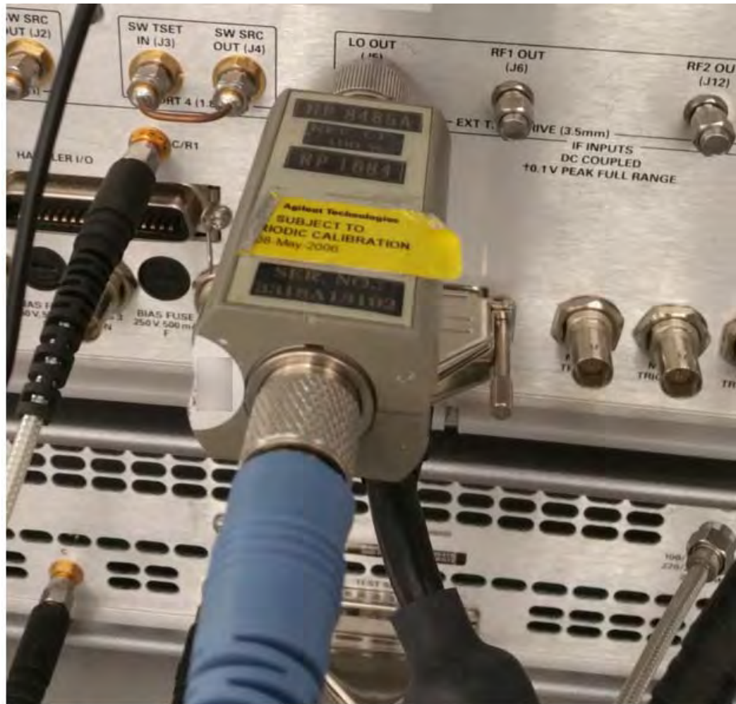
Figure 3-18 Connect Power Sensor to PNA Rear Panel LO
