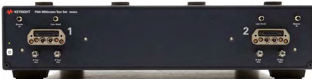
Figure 2-6 N5292A Option 400 (4-Port) Front Panel Features
