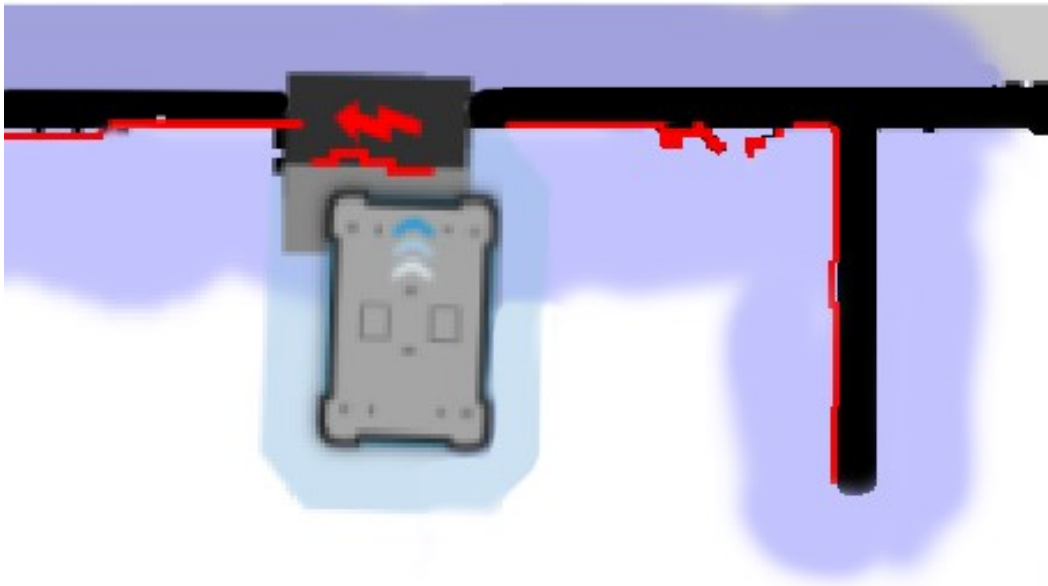
Figure 5.1. The red lines represent what the laser scanners detect. The robot is correctly localized when they align with the black lines that represent walls.
