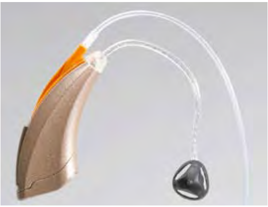
Figure 5. Probe tube attached to the Integrated Real Ear Measurement adaptor on a Zön hearing instrument.
