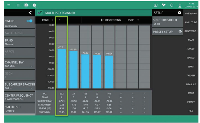
Figure 20. Field Master Pro MS2090A RTSA 5G Signal Scan Signal Causing Interference Outlined in Green Rectangle
