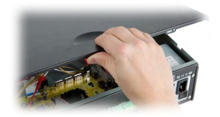
Using the thumb notch on the top of the unit, gently slide the cover about an inch to the rear of the unit, then lift it up. Once it is off, set the lid aside in a safe place where it won't get scratched.
