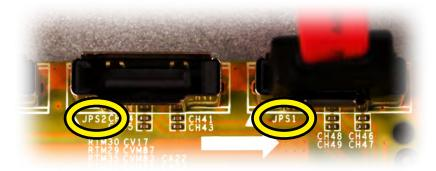
Using the extra SATA cables provided with the recorder, connect each hard drive to the mother board.
