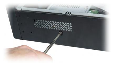
Remove the two black screws that hold the mounting bar in place. They are on the exterior of the unit, one at each side of the recorder.
