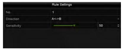
Figure 9. 5 Set Line Crossing Detection Rules
