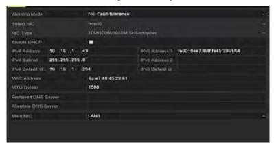
Figure 11. 2 Net Fault-tolerance Working Mode
