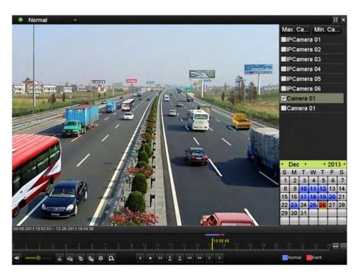
Figure 6. 8 Interface of Playback by Time
