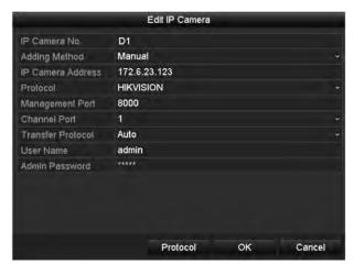
Figure 2. 31 Edit IP Camera Interface - Manual
