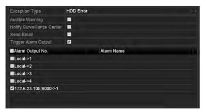
Figure 12. 23 Configure HDD Error Alarm
