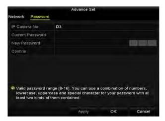
Figure 2. 26 Password Configuration of the Camera
