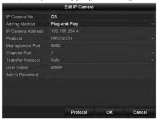
Figure 2. 30 Edit IP Camera Interface - Plug-and-Play
