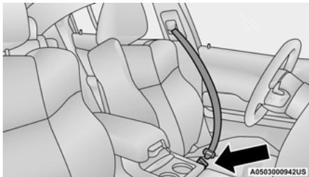
Inserting Latch Plate Into Buckle
