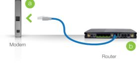
one end of the cable to your modem. Connect the other end of the cable to the blue
