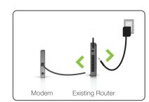
Power Off your Modem Remove Backup Battery Power off the modem by disconnecting the modem's power adapter from the power outlet. If your modem has a backup battery, remove the backup battery from your modem. Do NOT power on your modem until Step 4. Modem
