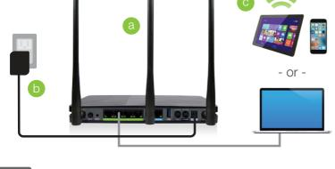
Attach the Power Adapter to the Router's **PWR** port and a power outlet.
