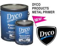
DYCO MP50 is a fast drying medium oil phenolic metal primer. MP50 incorporates zinc phosphate as its primary rust inhibiting additive. It cures rapidly to a tough, strong, solvent resistant film.
