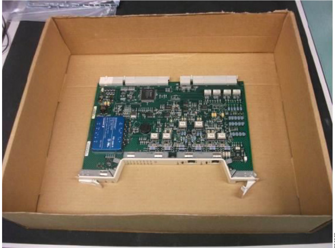
Figure 2-24 Failed Card Returned to Cisco in Inappropriate Packaging (without ESD-protective bag or foam to prevent mechanical damage during transportation)
