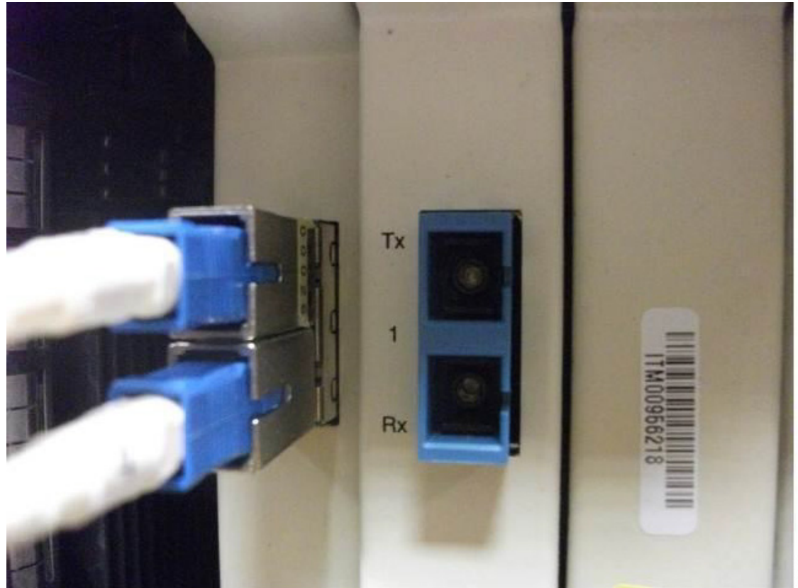
Figure 2-36 Another Example of Unused Optical Ports Without Protective Caps
