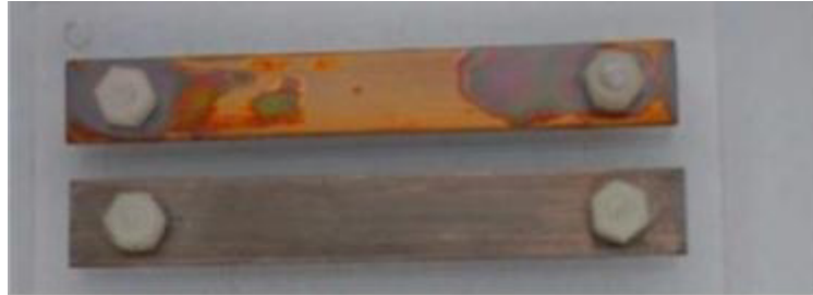
Figure 3-16 Copper and Silver Coupons Exposed to a G3 Classified Environment for 30 days
