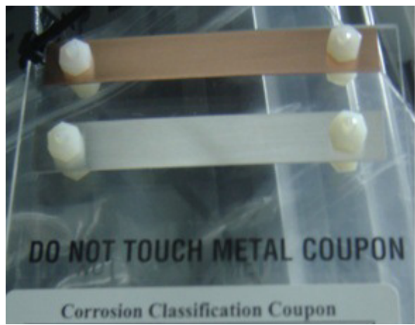
Figure 3-15 Copper and Silver Coupons used for Reactivity Monitoring of Corrosion
