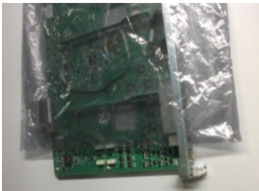
Figure 3-24 Board Stored in an Unsealed Antistatic Bag
