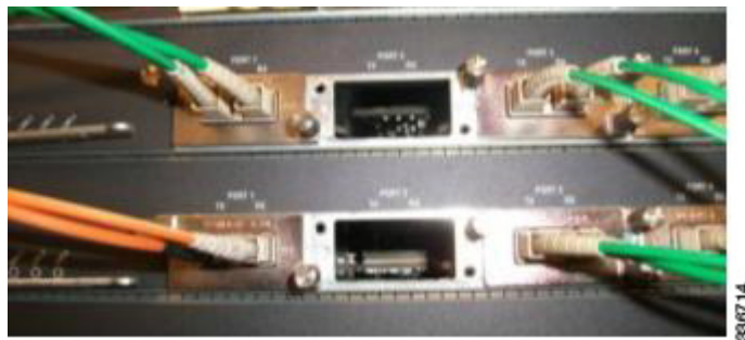
Figure 2-36 Another Example of Unused Optical Ports Without Protective Caps
