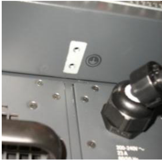
Figure 2-14 Missed System (NEBS) grounding on a Cisco Catalyst 6500
