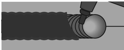
PARTIALLY CHIPPED AWAY TO SHOW WELD
