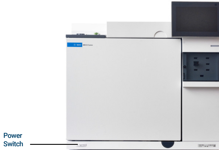
Figure 6. Power switch location
