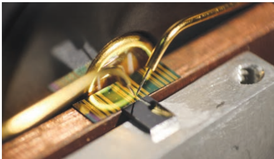
Semiconductor Laser Integrated on a Silicon Chip to power internet communications of the future. Photo credit: Zihao Wang
