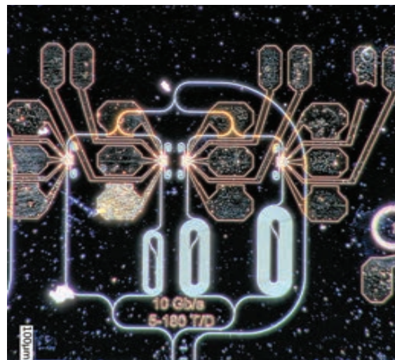
Photonics Circuit on a Silicon Chip that will be used to replace the power draining, slow, electrical wires we use today. Photo credit: Michael Fanto/Stefan Preble
