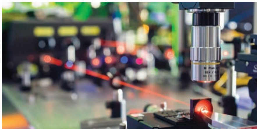
Future Photon Initiative: FPI spans the entire field of photonics from advanced optical systems down to photonic devices of the scale of nanometers. In this photo red laser light is directed into a chip (bottom right) with nanoscale photonic devices. Photo credit: Michael Fanto
