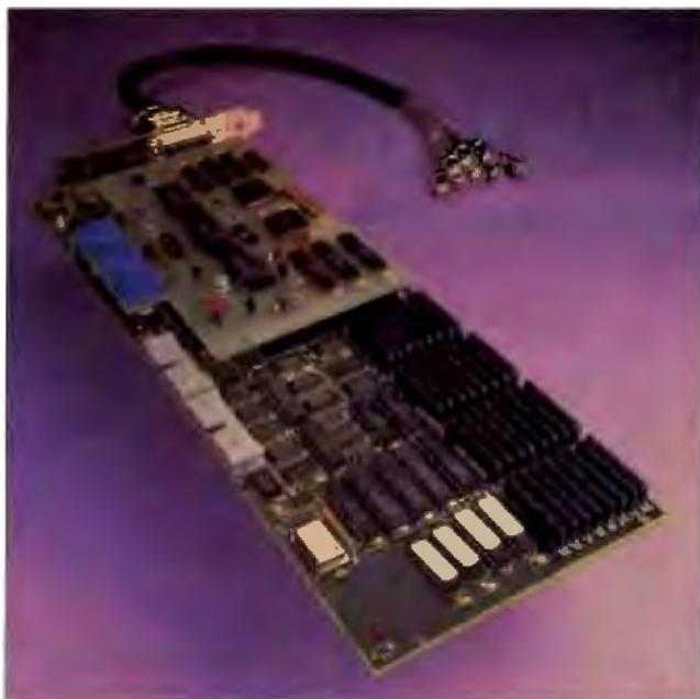
Capture color for real-time processing with the DT2871.
