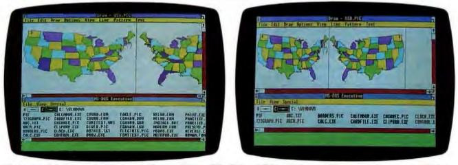
Photos 4 and 5: Microsoft's Windows 1.03 running under EGA (left) and VGA (right) modes illustrates the increased resolution that VGA offers.
