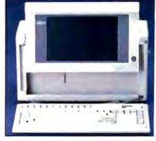
COMPAQ Portable 386 Model 40 80386 Processor 1 Megabyte RAM . 40 MB Fixed Drive 1.3 MB Diskette Drive No CQ114
