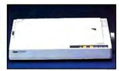
**STAR MICRONICS NX-15** · 120 CPS Draft. /50 CPS NLQ 5K Buffer, 132 Column Friction & Tractor Feed \$319 No. SGNX15
