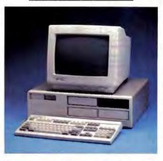
one 32-bit slot. You can provide the Z-386 with a maximum of 16 megabytes of RAM by filling the three remaining 32-bit slots with Z-515s and substituting another Z-515 for the Z-505 that comes with the basic system.
