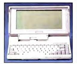
TOSHIBA T-1000 Lap Top Fully IBM compatible 512K RAM 720K 31/2" Disk Drive . e. 640 x 200 Pixels
