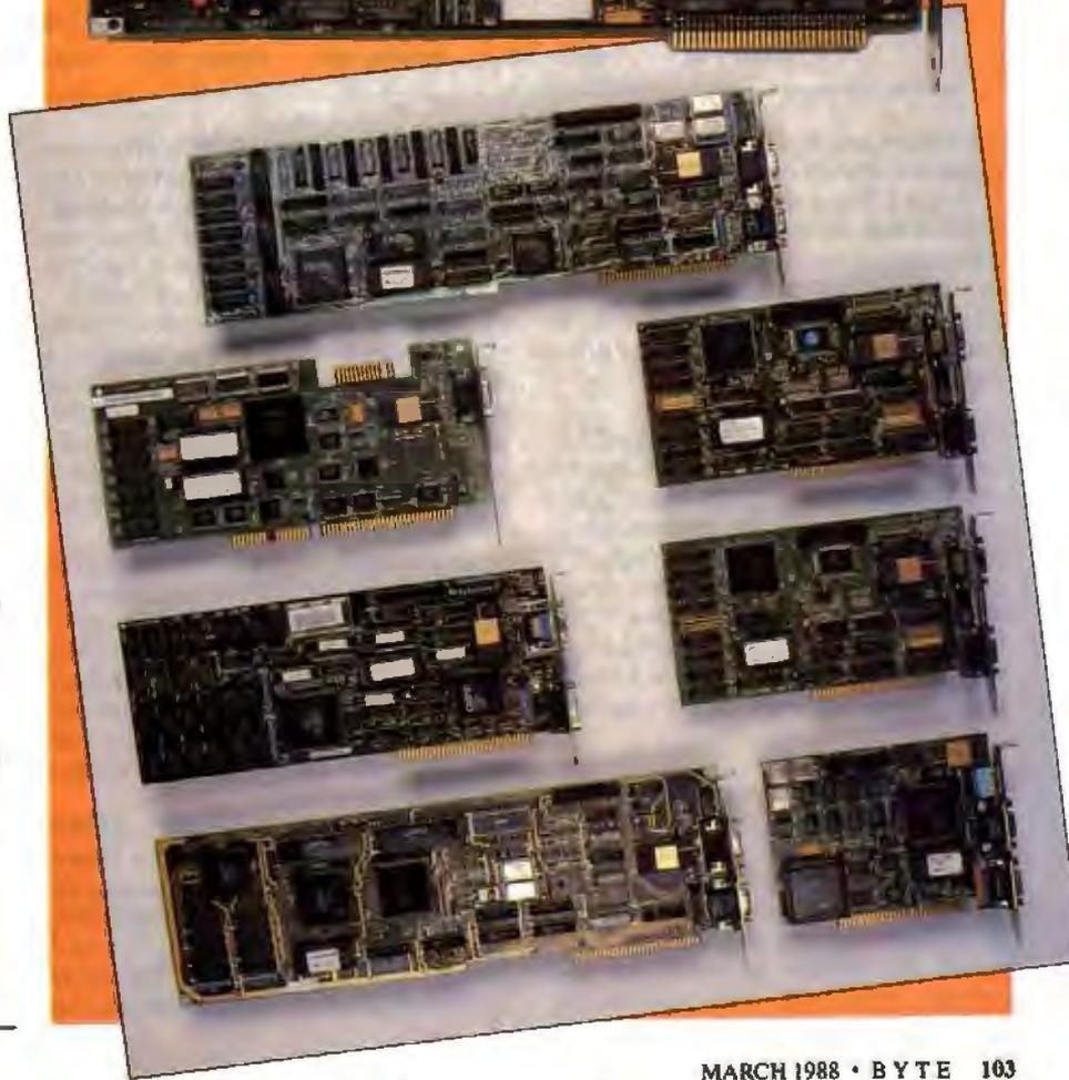
**Photo 1:** The NSI Smart EGA Plus, Thomson Enhanced Graphics Adapter Ultra Version, Paradise Autoswitch EGA480, and Quadram Quad ProSync! are typical of the half-slot enhanced EGA boards.
