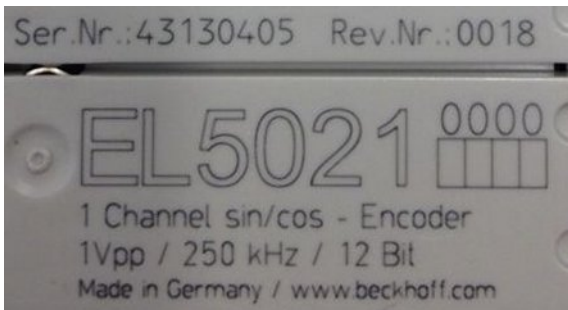
Fig. 136: EL5021 EL terminal, standard IP20 IO device with serial/ batch number and revision ID (since 2014/01)
