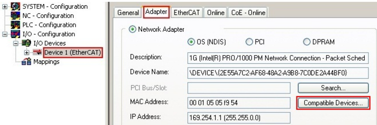
Fig. 156: EtherCAT device properties(TwinCAT 2): click on “Compatible Devices...” of tab “Adapte””
