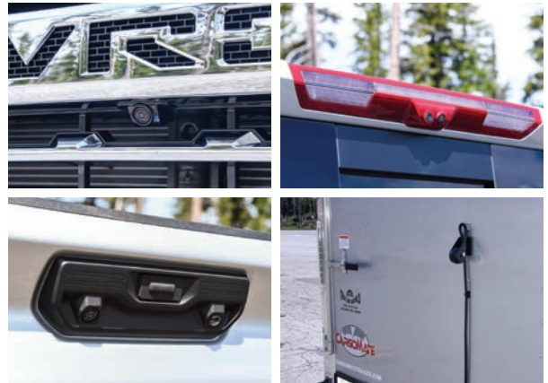
Ⓢ Clockwise from top left: The front camera is angled downward slightly to assist with parking or spotting obstacles when driving off-road. Two cameras mounted in the Center High Mounted Stop Lamp (CHMSL) provide a high rear view and bed view. A GM accessory camera can be mounted to the rear of the trailer to provide crystal-clear views of what’s directly behind you. A tailgate camera (left) and small light make backing and hitching a travel trailer a one-person job.
