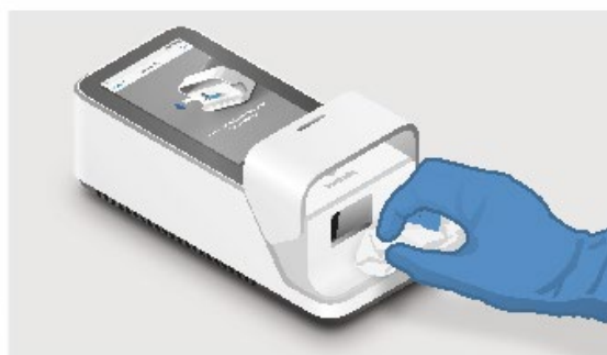
Cleaning the area around the Test Strip slot
