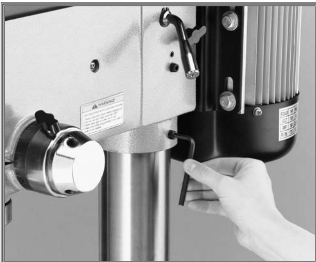
Figure 16. Tighten setscrews to secure headstock.
