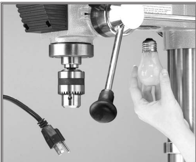
Figure 17b. Installing a light bulb.
