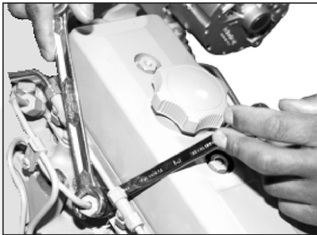
FIGURE 24. BLEEDING THE INJECTOR LINES
